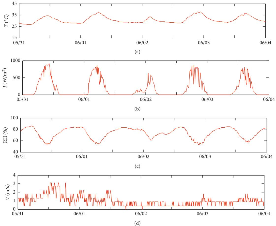
FIGURE 5: Weather data during the experiment: (a) air temperature, (b) global horizontal solar radiation, (c) relative humidity (RH), and (d) wind speed at 1.8 m height.
