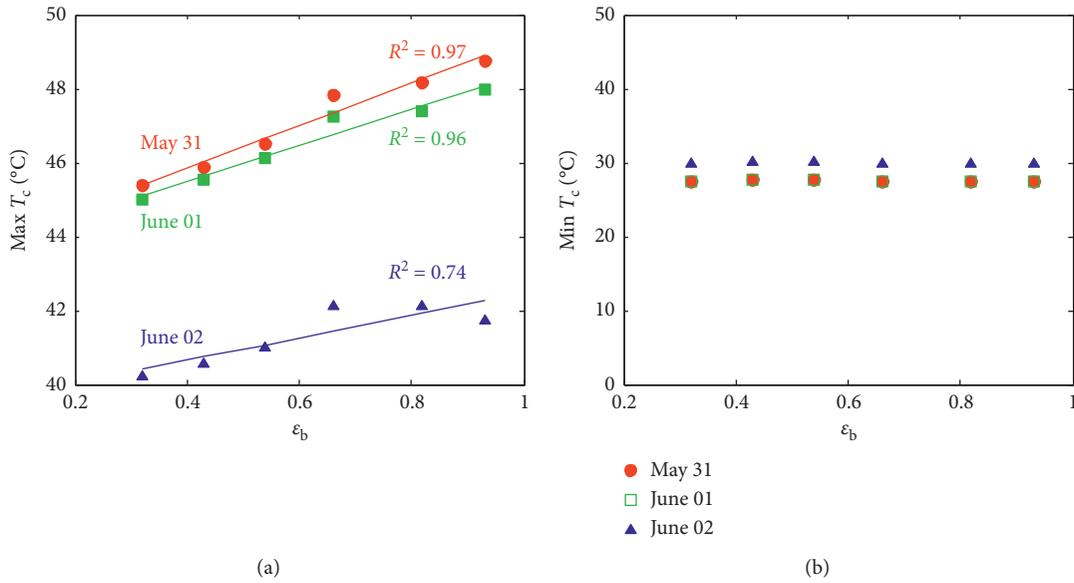
FIGURE 10: Daily maximum ( $\text{max } T_c$ ) and minimum ( $\text{min } T_c$ ) temperatures at the ceiling: (a)  $\text{max } T_c$  and (b)  $\text{min } T_c$ .
