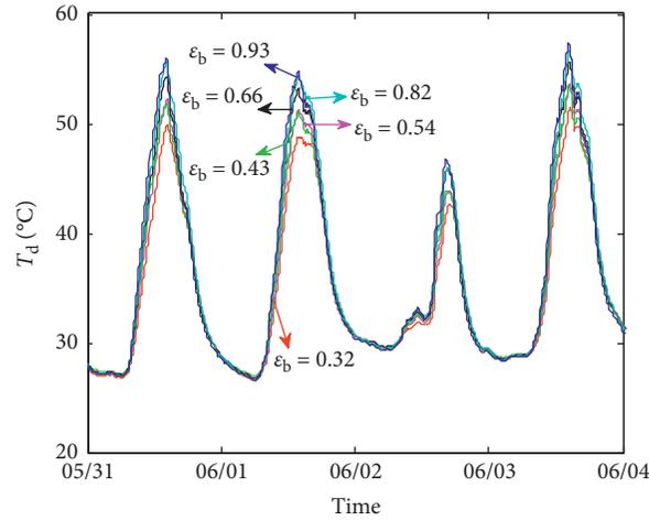
FIGURE 7: Temperatures of decks below the tiles with different  $\epsilon_b$  values.
