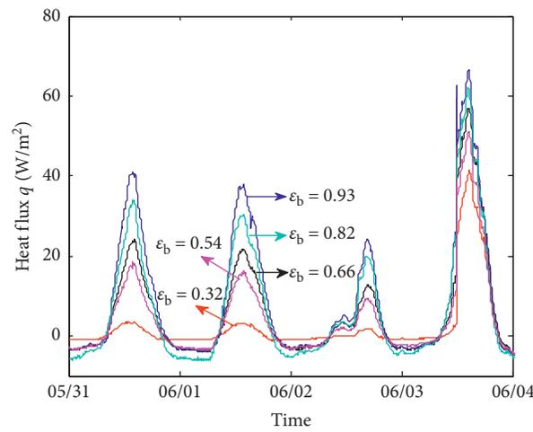
FIGURE 11: Heat fluxes at the ceiling are controlled by the tile's underside emissivity.
