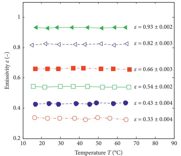
FIGURE 3: The emissivity of samples coated with different emission latexes. The emissivity is independent of temperature.
