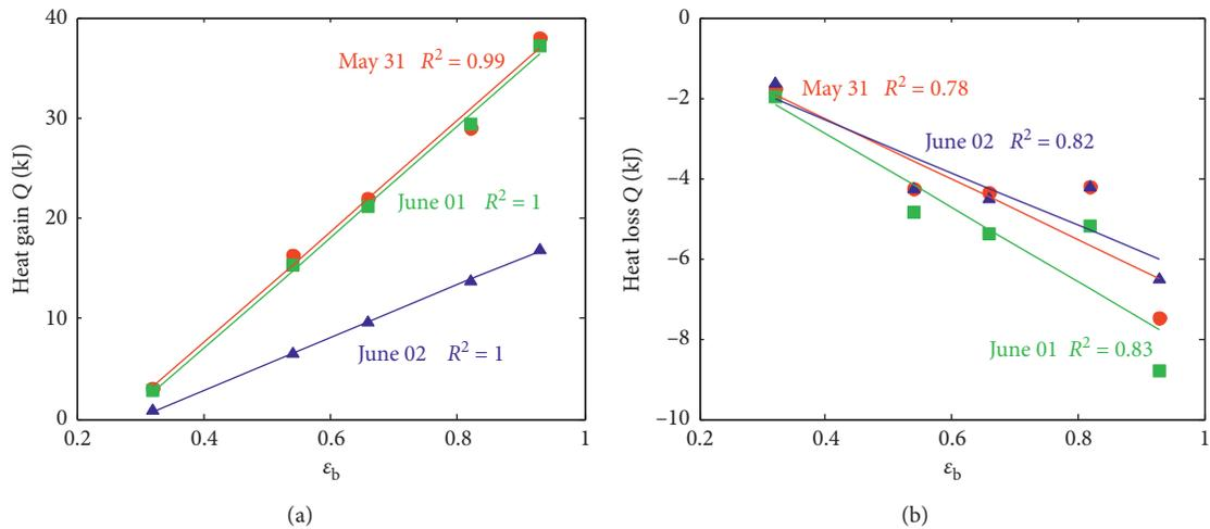
FIGURE 12: Daily cumulative heat gain/loss at the building ceiling varies linearly with emissivity: (a) heat gain versus  $\epsilon_b$  and (b) heat loss versus  $\epsilon_b$ .
