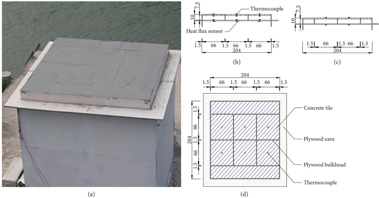
FIGURE 2: The experimental building cell and the deployment of measurement sensors on the concrete roof tile. (a) A photo of the roof, (b) roof's front view, (c) roof's side view, and (d) roof's plan view.
