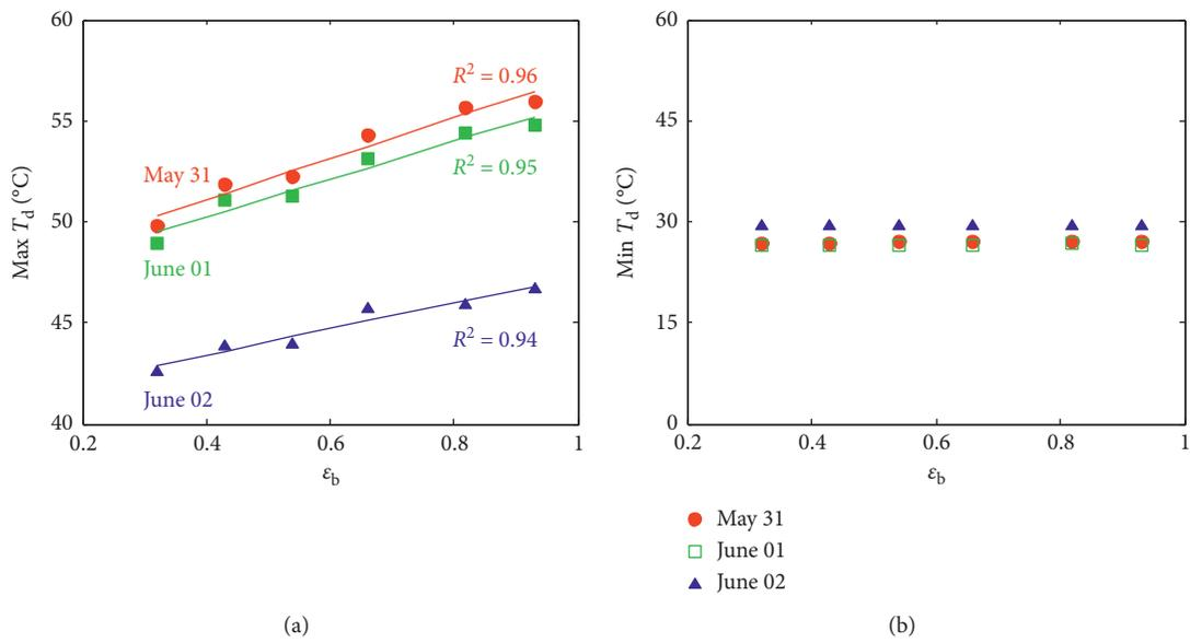
FIGURE 8: Daily maximum ( $\max T_d$ ) and minimum ( $\min T_d$ ) temperature at the roof deck: (a)  $\max T_d$  and (b)  $\min T_d$ .
