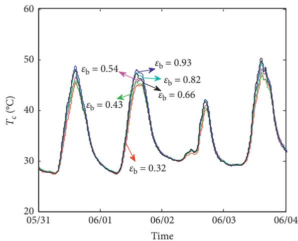
FIGURE 9: Temperatures of the ceilings under concrete roof tiles with different  $\epsilon_b$  values.
