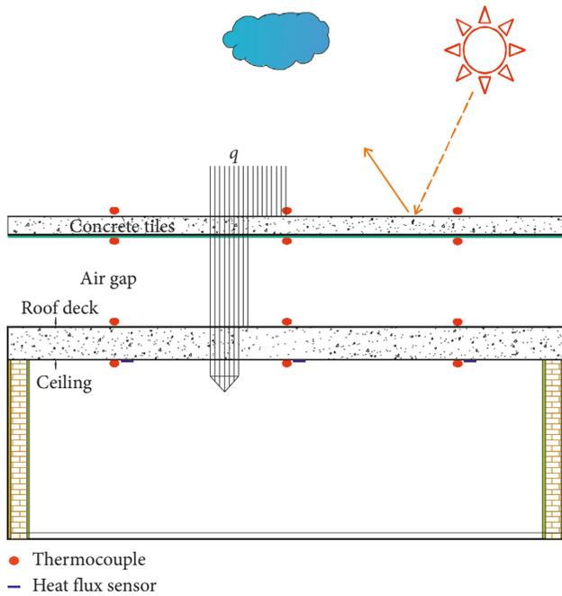
FIGURE 4: Sensors are deployed at different heights of a concrete tile roof to log the local temperature and heat flux.
