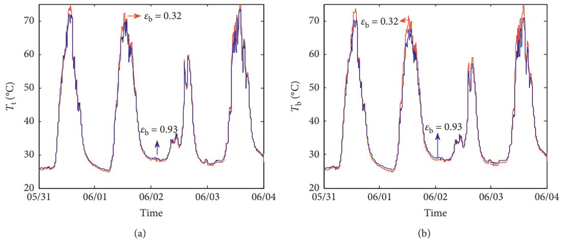
FIGURE 6: Tile's temperatures during the experiment: (a) rooftop temperature and (b) tile's underside temperature.
