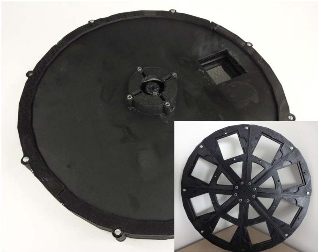
**Figure 2.3.6.** Automated filter wheel switcher
