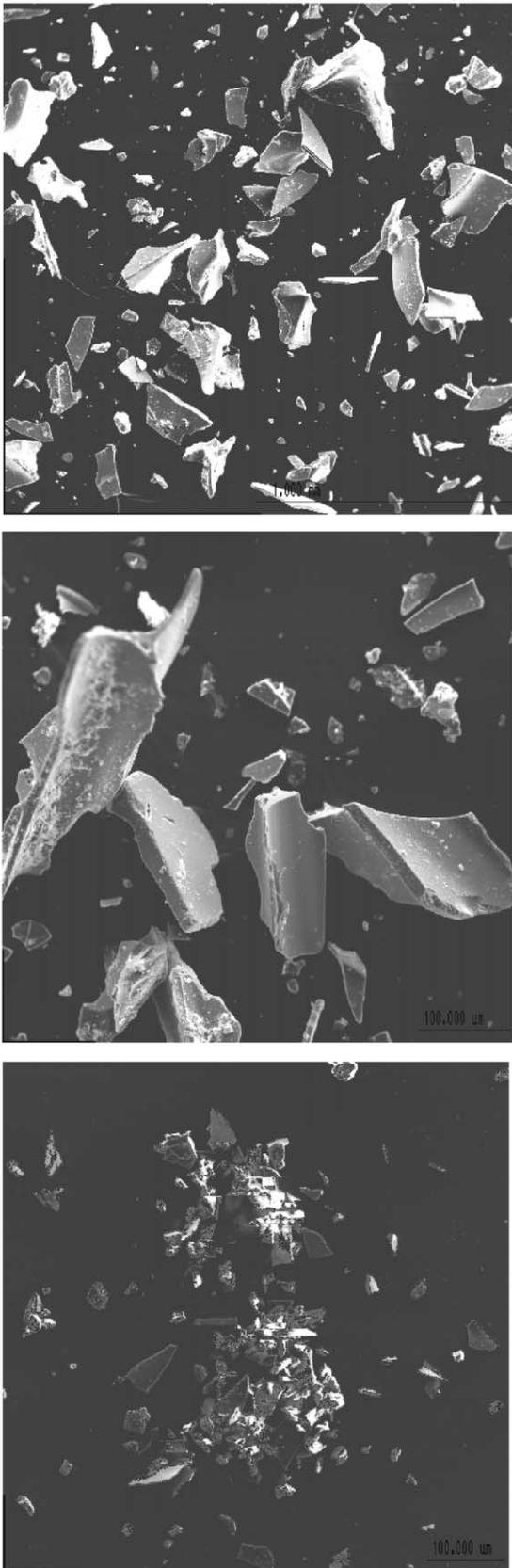
**Figure 2.** Scanning electron microscopy images of the Broadwater ash sample from Western Nebraska showing the overall shapes of all the ash samples in this study. We interpret these as bubble wall shards. The image at the top illustrates the spontaneous aggregation of these ash particles that occurs in the Roller Analyzer during elutriation.
