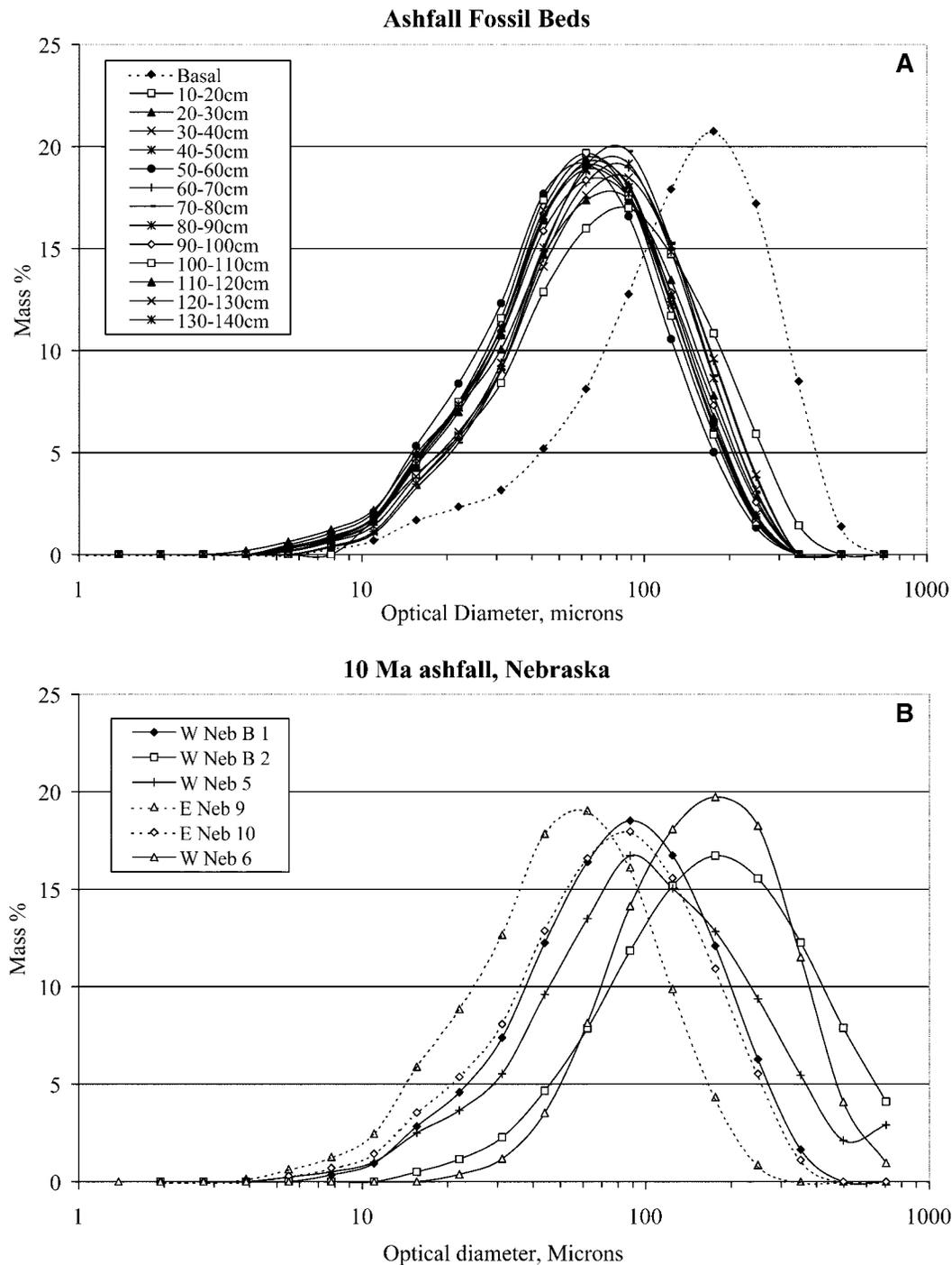
**Figure 3.** Optical diameter size distribution data for Nebraska 10-Ma ashfalls as determined by Microtrac laser diffraction. *A*, Data for a stratigraphic section collected at Ashfall Fossil beds in NE Nebraska; *B*, size differences between the localities in northeastern (*dashed lines*) and western Nebraska (*solid lines*).
