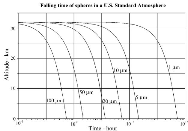
**Figure 7.** Fall times for spherical particles with a density of 2300 kg/m<sup>3</sup> from 32 km in the atmosphere.
