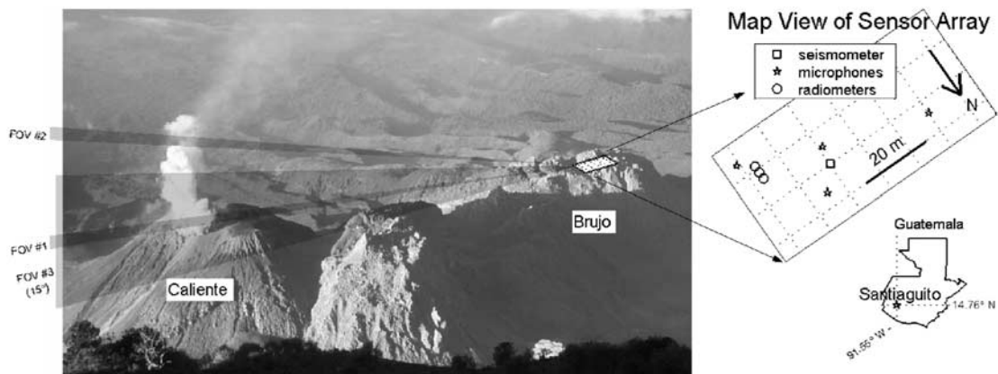
Figure 1. Santiagouito dome viewed from Santa Maria. Active Caliente vent is at left (east) \sim 1600 m from the inactive Brujo Dome, where sensors (inset map) were installed. Thermometer FOVs are shown as transparent cones.
