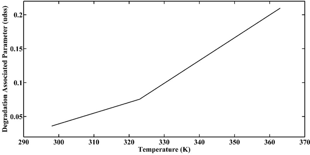
**Fig. 2** Degradation associated parameter  $u_{dss}$  against temperature
