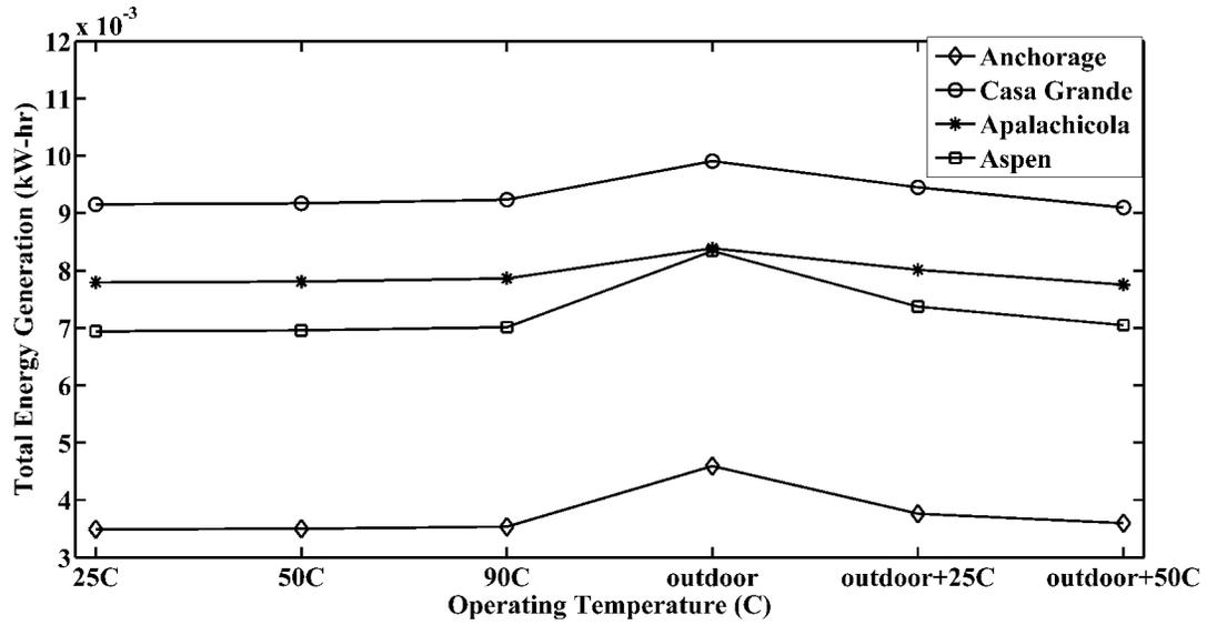
**Fig. 15** Maximum electricity generation over a year for the four cities at sustained temperature (anneal cycle is one time per day) and outdoor operating conditions (anneal cycle varies from one place to another)
