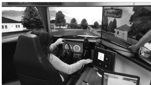
Figure 2: Driving simulator setup, visual display monitor with webcam, and LEAP Motion.
