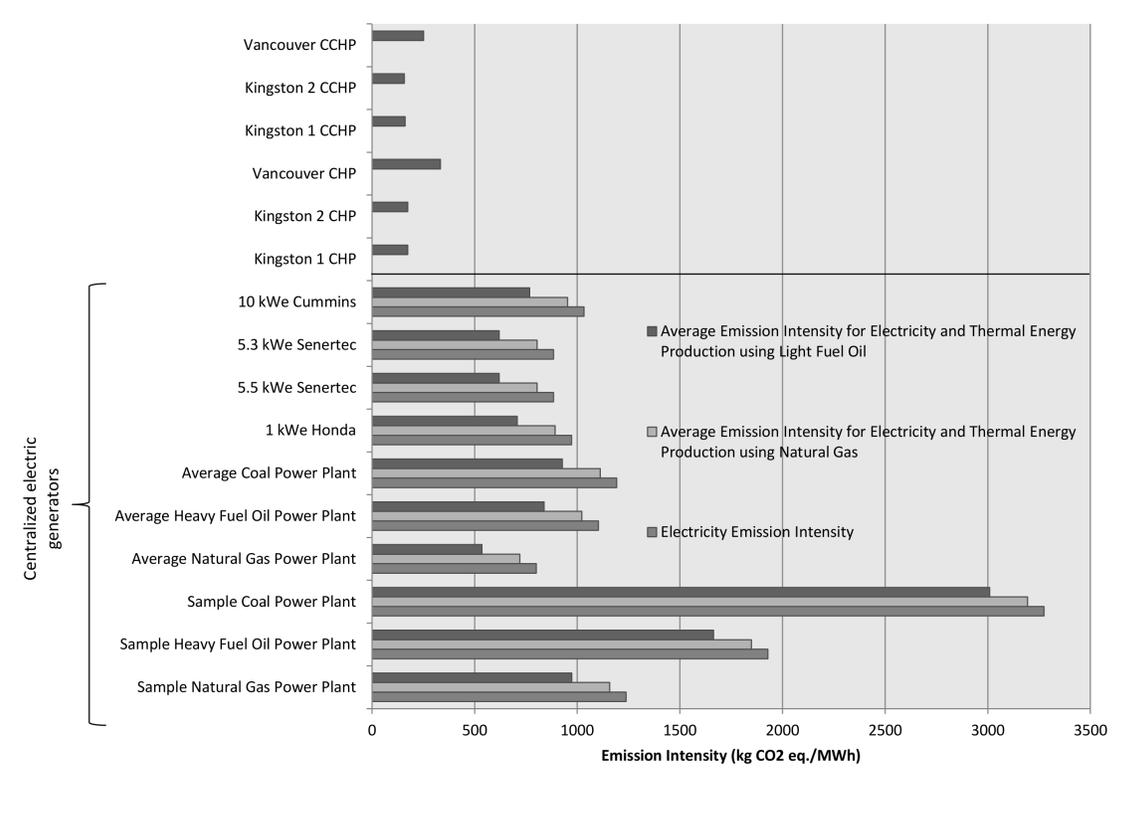
Figure 6. Emission intensity comparison for PV-CHP, PV-CCHP, and centralized systems for select case studies to meet all end-uses (both thermal and electrical). The average emission intensities are for on site electrical and thermal energy production.
