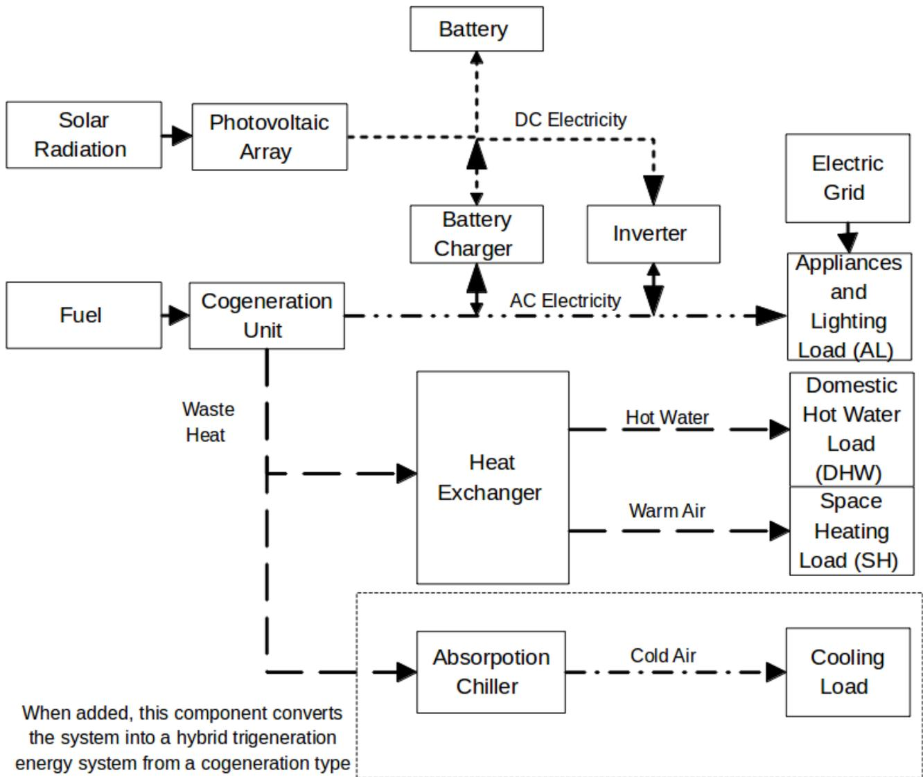
Figure 3. Energy flow of hybrid PV-Cogen/Trigen system.
