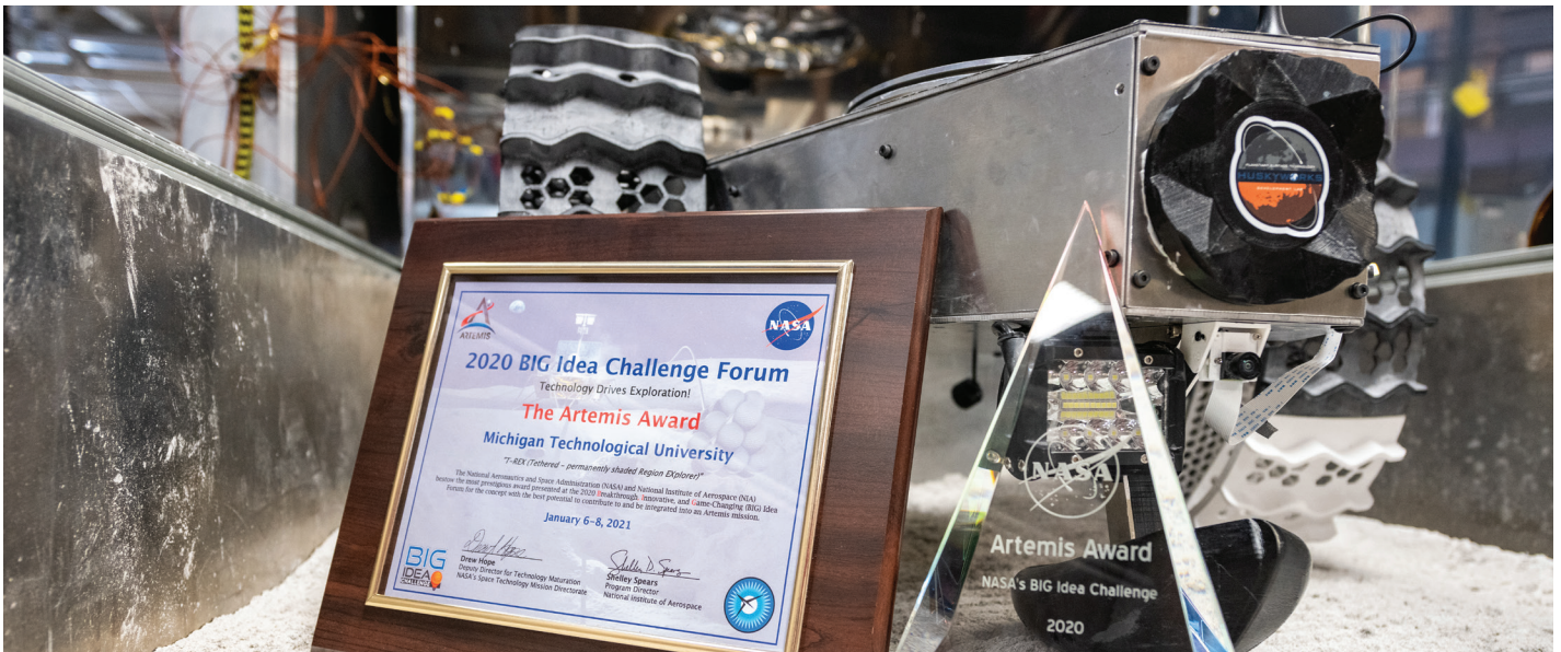
BIG Idea teams took on near-term technology capability requirements to support NASA's exploration objectives for permanently shadowed regions (PSRs) in and near the moon's polar regions. T-REX, short for the Tethered permanently-shadowed Region Explorer, is MTUEngineering's award-winning prototype designed to lay down lightweight, superconducting cable connected to a lander. Once the rover reaches its final spot after traversing rocky crater terrain into the PSRs, the rover can serve as a recharging hub and communication relay for other robots, providing continuous power without direct sunlight.
