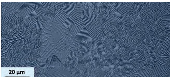
A Zn-3Mn eutectic alloy, showing Mg<sub>2</sub>Zn<sub>11</sub> in a spiral pattern within the hcp Mg matrix. Optical micrograph by Ehsan Mostaed, MSE postdoctoral assistant.
