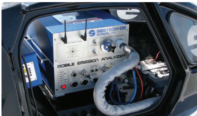
Mobile emissions analysis system collects emissions and fuel consumption data while the vehicle is "in-use."
