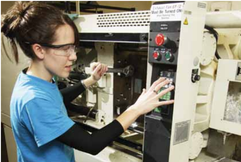
Colleen installs a die on a plastic extrusion machine in the IDM Lab.
