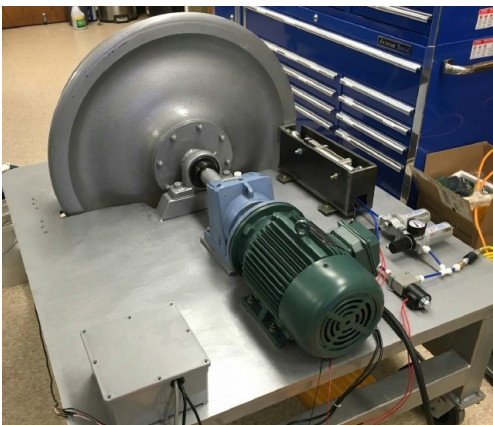
Hump Yard Sensor Test Stand
