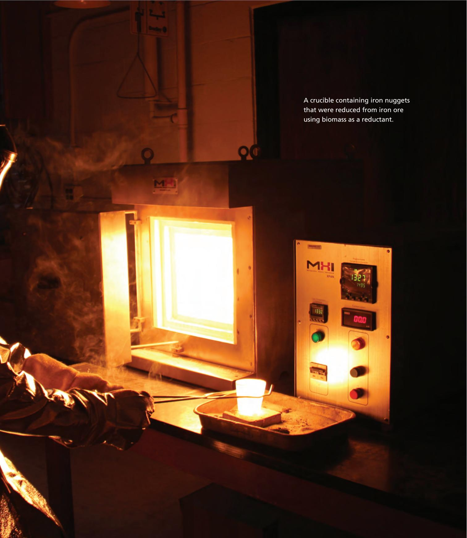
A crucible containing iron nuggets that were reduced from iron ore using biomass as a reductant.
