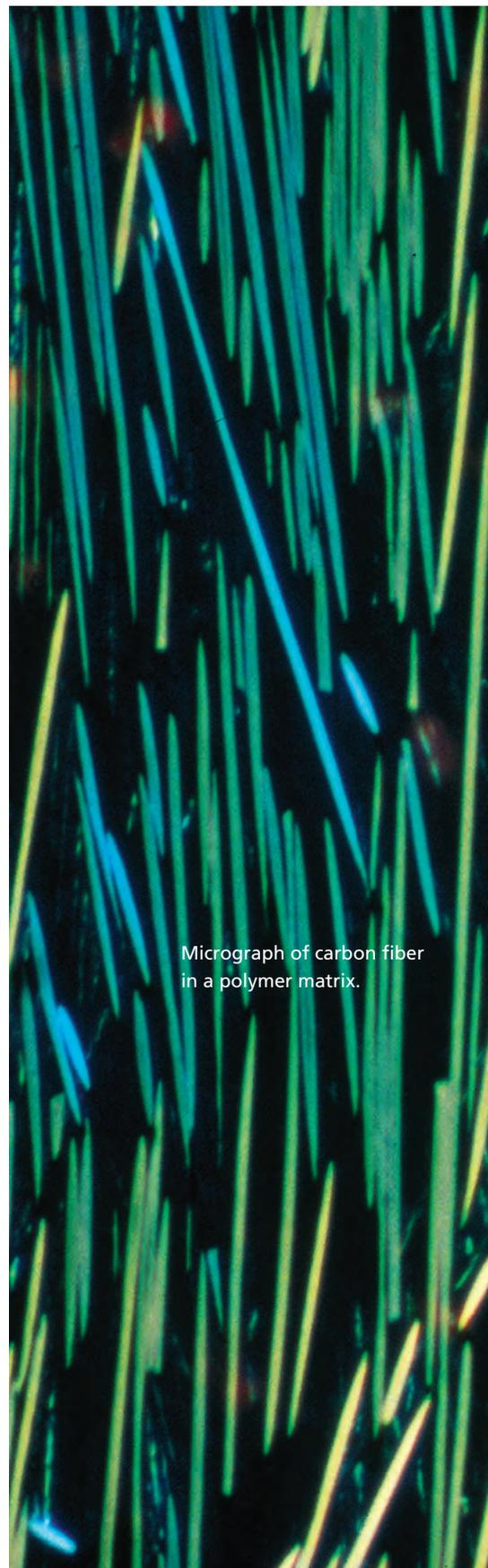
Micrograph of carbon fiber in a polymer matrix.
