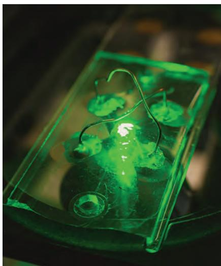
Fluorescent illumination of an microfluidic device. Wires serve as electrical contacts to manipulate cells within the microchannels.
