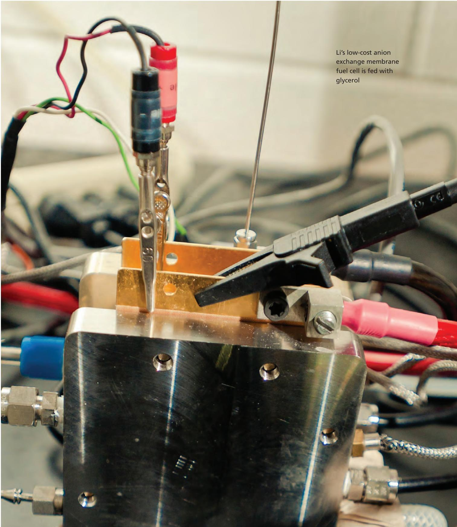
Li's low-cost anion exchange membrane fuel cell is fed with glycerol
