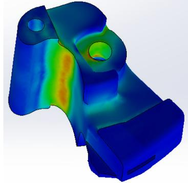
Finite Element Model of Type E Coupler
