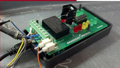
Locomotive Sand Sensor Prototype
