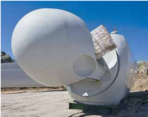
Front view of a windmill rotor hub, with nacelle behind
