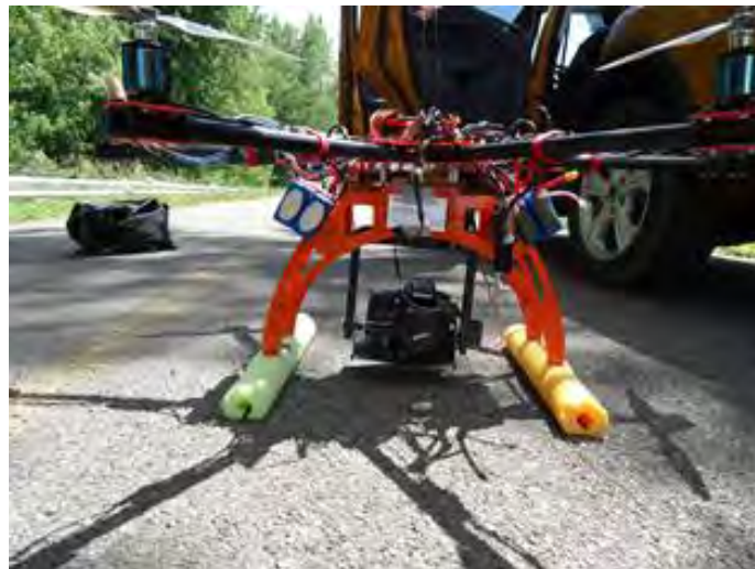
Figure 40: The Nikon D810 attached to the Bergen Hexacopter.
