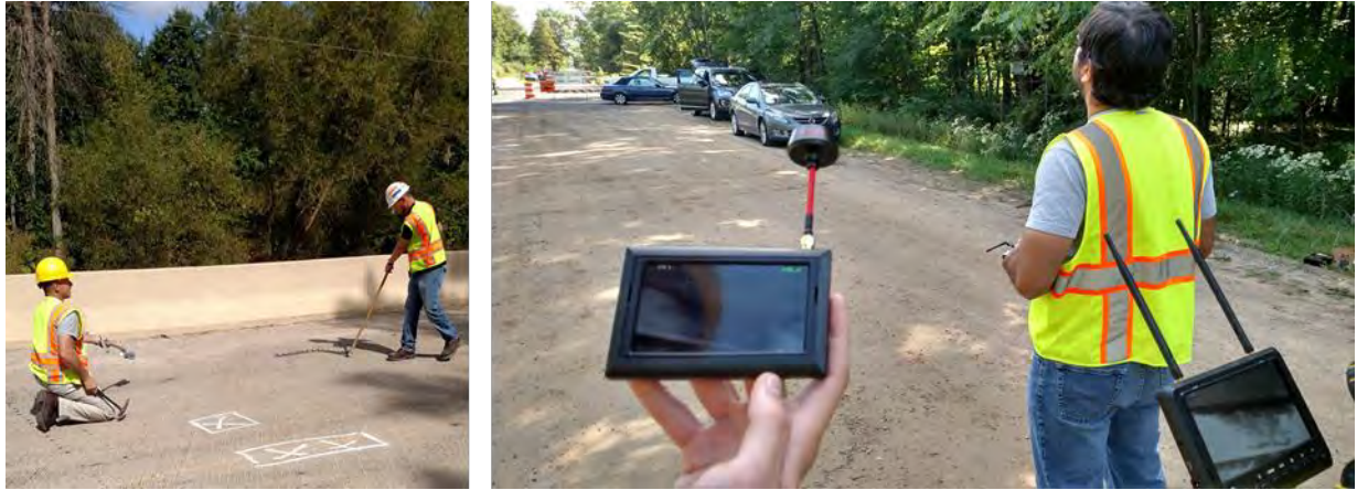
Figure 3: Gordonville Road data collection photos: MDOT staff collect ground truth delamination data with chain dragging (left); R. Dobson collects thermal data with the Bergen hexacopter and FLIR Vue Pro combination with real-time display of the thermal data visible in two first-person viewer screens (right).
