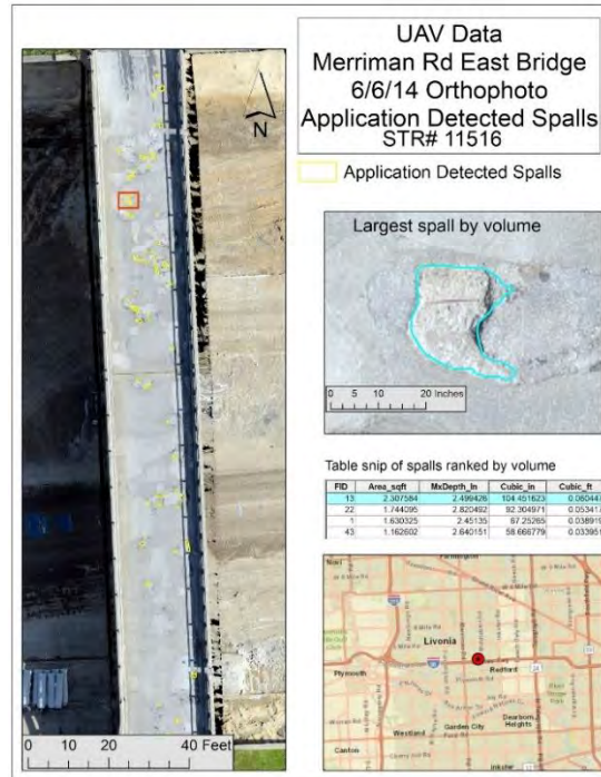
Figure 78: Spall layer of the Merriman bridge with close-up of the largest spall by volume selected from the attribute data.
