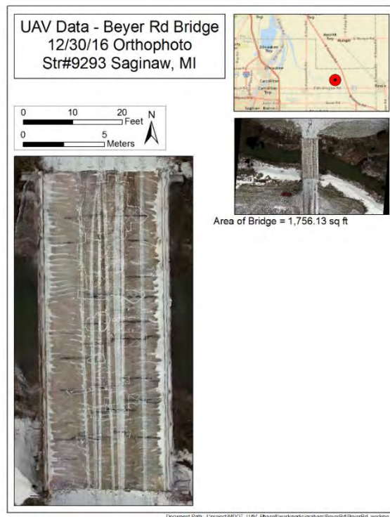
Figure 16: Beyer Road Bridge, with delamination markings from a MDOT sounding survey.
