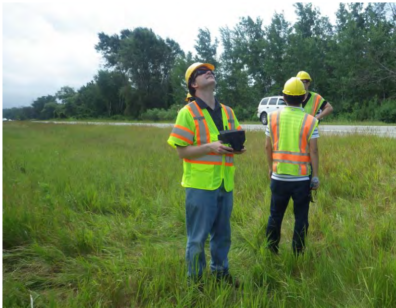
Figure 24: Example of operating the Mavic Pro safely from the US-31 right-of-way; the operator is looking towards the UAV while also using the FPV screen to enable live viewing of what the UAV is seeing while it collects imagery and video data.
