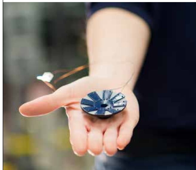
Triangular sensors form a polar array, exposing the sample to all eight sensors.
