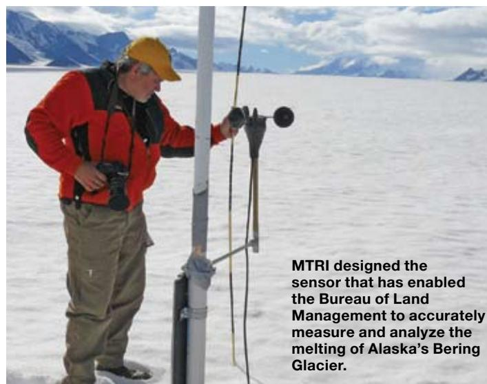
**MTRI designed the sensor that has enabled the Bureau of Land Management to accurately measure and analyze the melting of Alaska's Bering Glacier.**
