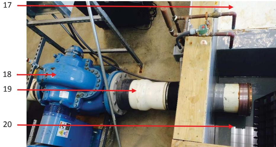
**Figure 7:** Plan view of the pump and water channel (outlet section) setup. *List below indicates feature details.* (Image by author, 2015)
