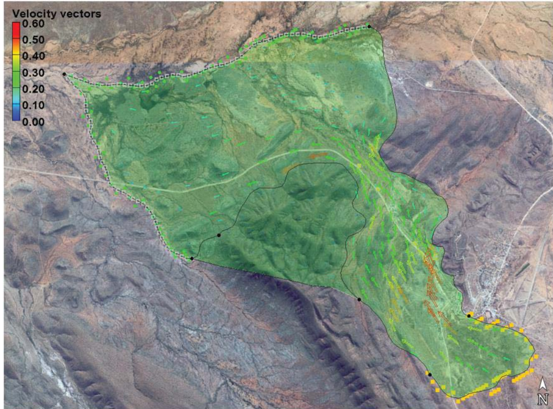
Figure 19: Preferential flow through alluvial soils in model (m/day) (approximate scale 1cm:700m)
