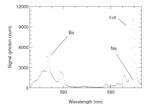
Figure 6: TRELIBS spectrum of calibration sample with additives of barium sulfate and sodium bismuthate. The sodium doublet is obscured by the iron peak.
