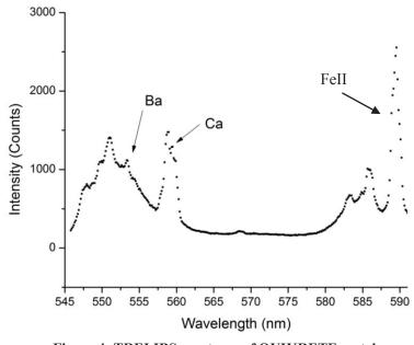
Figure 4: TRELIBS spectrum of QUIKRETE matrix
