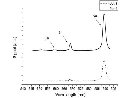
Figure 2: Evolution of TRELIBS spectral features with time delay of 15µs (top, solid line) and 30µs (bottom, dashed line).
