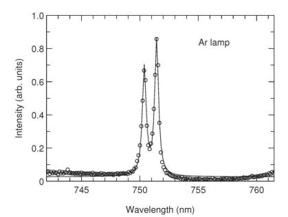
Figure 9: Spectrograph resolution determined by Argon lamp. Experimental data is indicated by the circles, and the data fit is indicated by the sold line.
