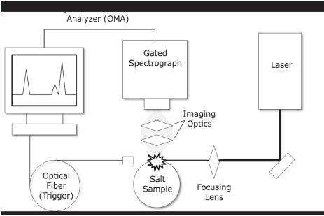
Figure 1: Optical tabletop TRELIBS setup.
