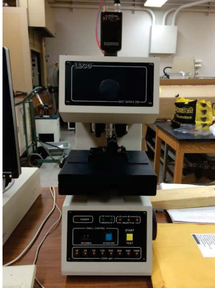
Fig. 3-3: LECO MHT Series 200 Vickers microhardness tester
