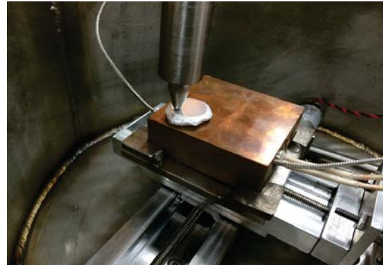
Fig. 3-4: Vickers macroindenter with a motorized copper heating block for elevated-temperature hardness testing.
