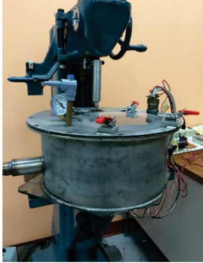
Fig. 3-4: Vickers macroindenter with a motorized copper heating block for elevated-temperature hardness testing.
