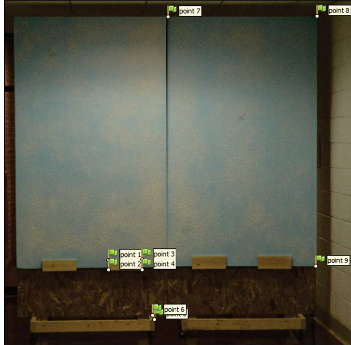
Figure 1-3 Laboratory scale model with the reference points used for registration.
