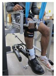
Figure 1. Anklebot mounted to the chair for testing the mechanical impedance in the medial/lateral rotation
