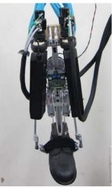
Figure 20. Measurement of the prosthetic foot mechanical impedance using the Anklebot
