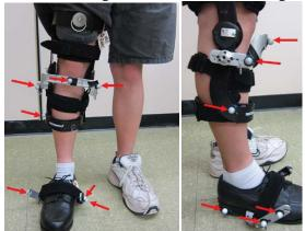
Figure 9. Knee brace and shoe with reflectors. The arrows point to the visible reflectors.
