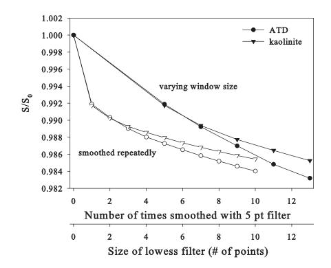
Figure 6. ATD and Kaolinite  $S/S_0$  for both number of times smoothed with 5 point window (hollowed circle and triangle) and 5 to 13 window size (filled circle and triangle) by AFM data
