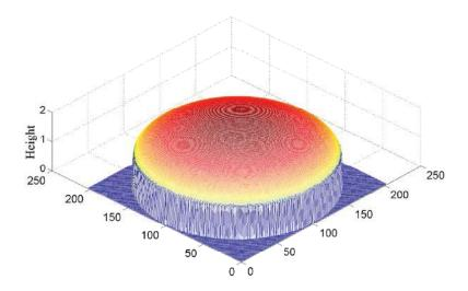
Figure 5. we set oblate spheroid major axis R= 10, resolution of AFM 0.1, and the aspect ratio (major axis / minor axis) is 10 which results in a  $\Delta$ S of 10%
