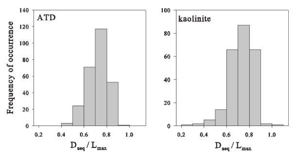
Figure 3. Histogram plots of  $D_{aeq}/L_{max}$  by SEM detected particles.
