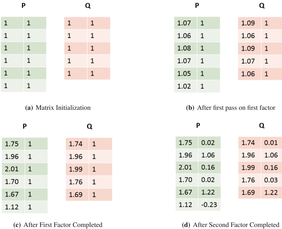
Figure 3.5: PQ Decomposition of Example Data
