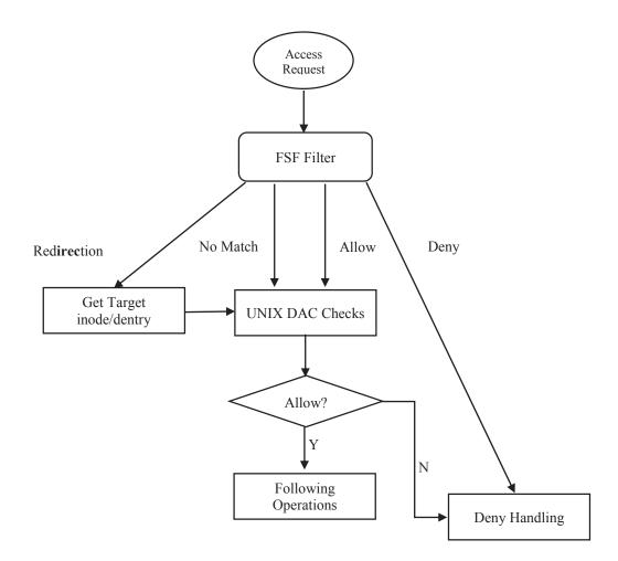
Figure 2: Work Flow of FSF
