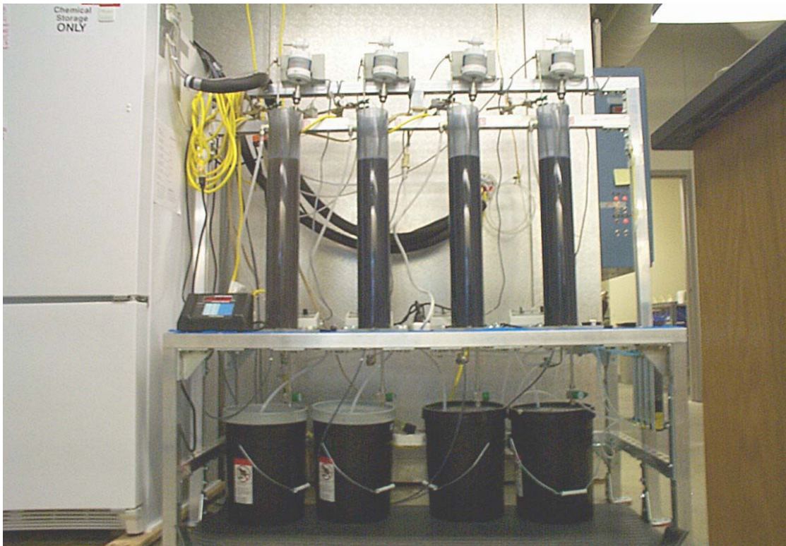
Figure 2.2 – Laboratory Set-up of Room Temperature SBRs: SBR5 to SBR8 (Left to Right); Refrigerator for Feed and Decant Storage (Left); Emergency Overflow Buckets (Bottom).
