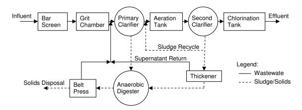
Figure 3. Activated Sludge Treatment
