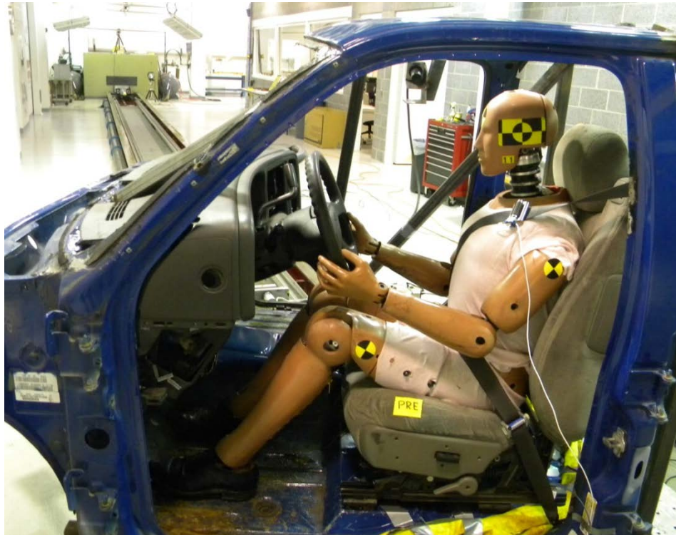
Figure 5.1. Sled test setup for 70° PDOF with an SUV
