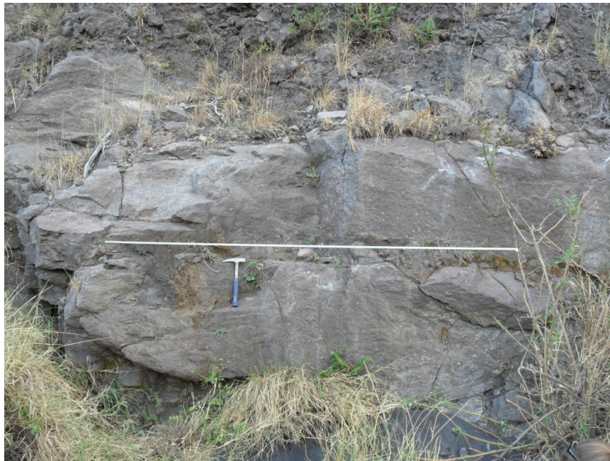
Figure 2-4 A horizontal segment using the scan-line approach.
