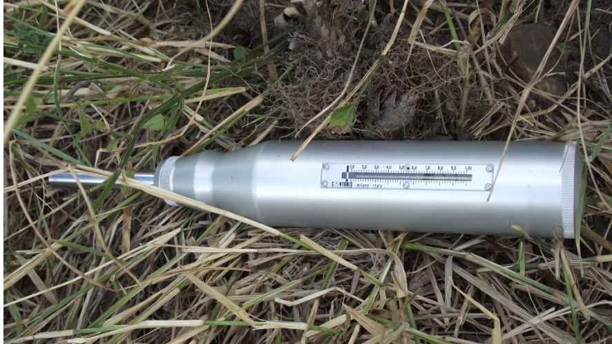
Figure 2-6 The Schmidt hammer measures intact rock strength in the field.
