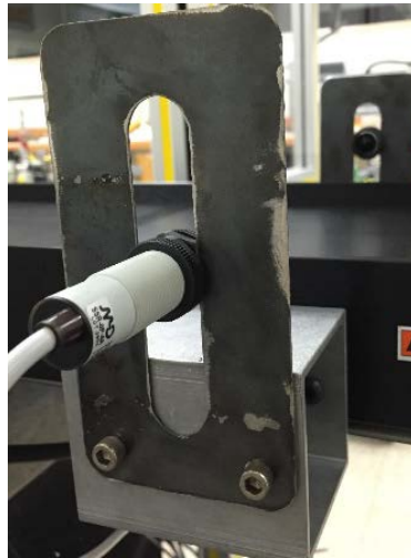
Figure 3. Through beam sensors mounted on brackets
