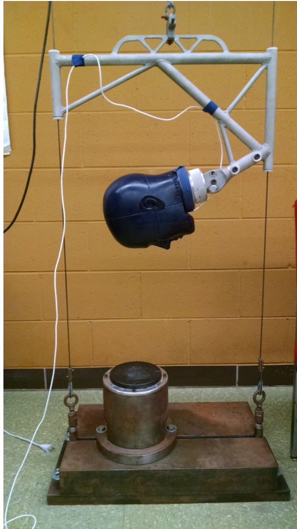
Figure 3-1 NOCSAE Standard Drop Tester at MTU based upon NOCSAE Standard Drop Test Equipment [9]
