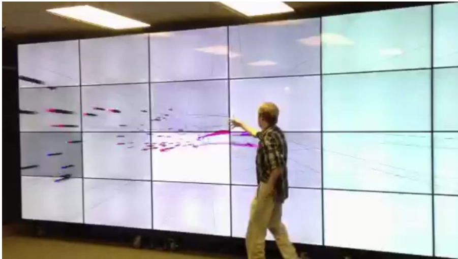
Figure A.7. Users can improvise real-time sonification and visualizations based on their location, movements, and gestures. They can change multiple mappings with a special-purpose scripting language.
