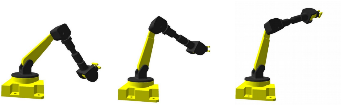
Figure A.13. A series of images showing the robotic arm moving the end effector up in world coordinates using my Inverse Kinematics implementation.
