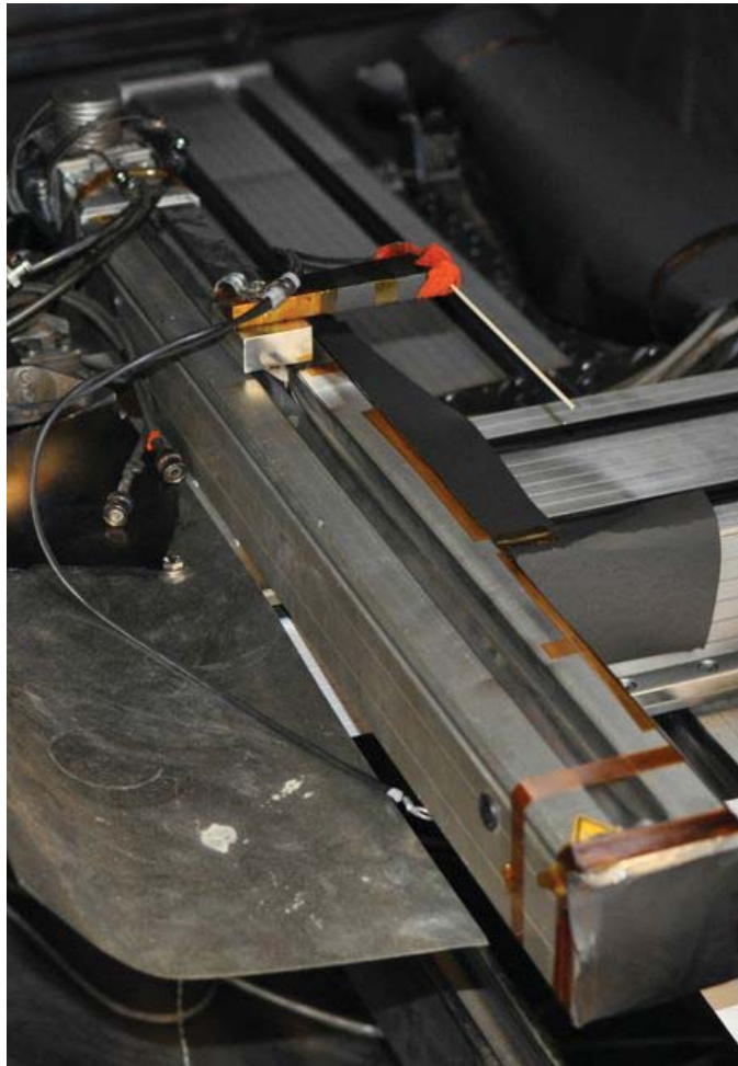
Figure 5.2: Assembled high-speed motion table with mounted double Langmuir probe
