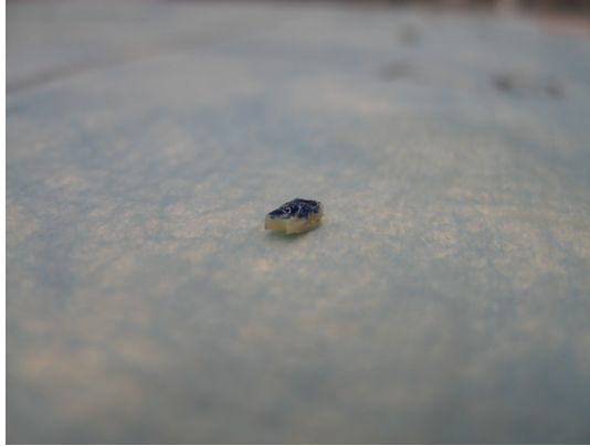
Figure A.3: Specimen painted with nail polish on the surface opposite to the surface being indented.
