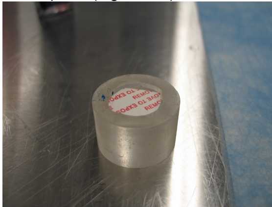
Figure A.4: Well-puck with double sided tape cut and inserted into it.
