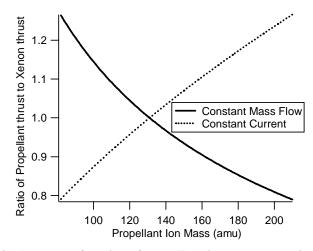
Figure A-1: Change in thrust as a function of propellant ion mass, assuming constant acceleration voltage
