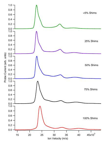
Figure 6-19: ExB probe traces taken as the level of shim current was varied. Data are for 400 V on the anode and 4 mg/s of xenon
