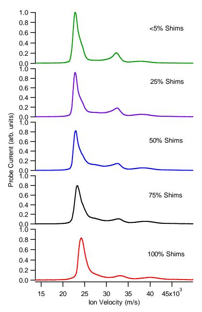
Figure 6-7: typical set of ExB probe traces taken as the level of shim current was varied. Data are for 400 V on the anode and 4 mg/s of xenon
