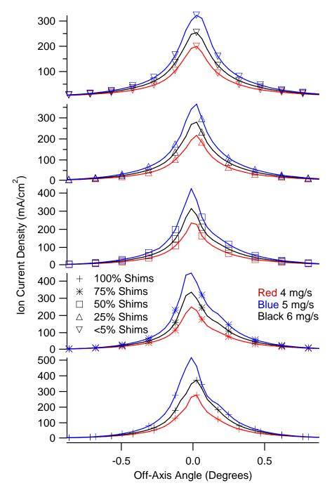
Figure 4-4: Beam Profile s with 400 V on the anode at all mass flows and levels of discharge current heating
