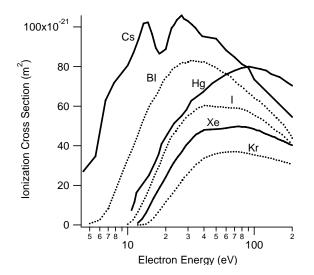
Figure A-3: Electron-Impact Ionization Cross Sections for bismuth, cesium, iodine, krypton, mercury, and xenon between threshold and 200 eV
