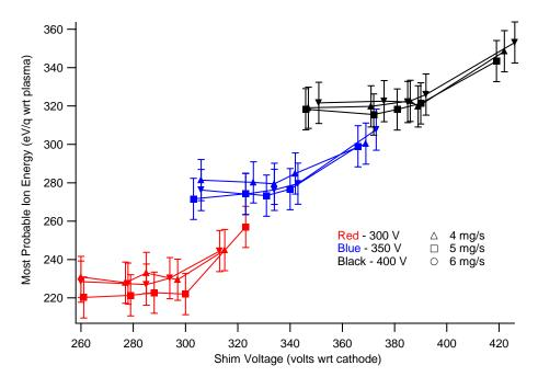
Figure 5-10: Most Probable Ion Energy as a function of all three experimental factors. Higher shim voltage indicates a higher proportion of discharge current on the shims.
