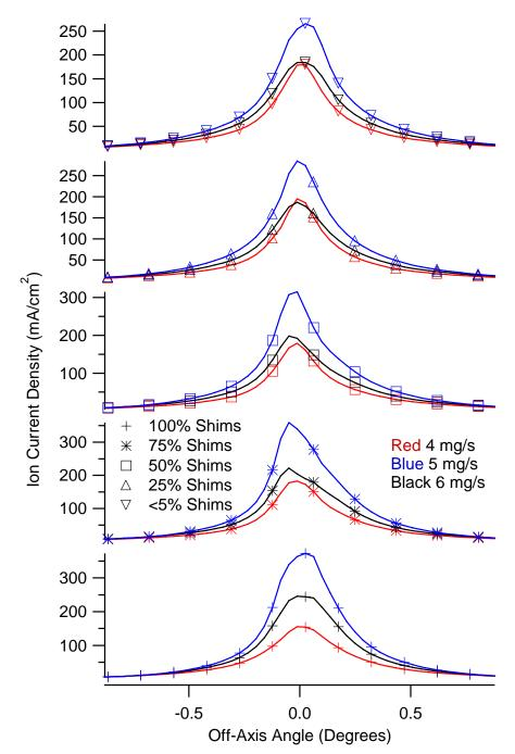
Figure 4-2: Beam Profiles with 300 V on the anode at all mass flows and levels of discharge current heating
