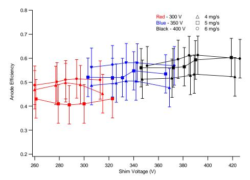
Figure 3-12: Thruster Efficiency as a function of all three experimental factors. Higher shim voltage for a given anode voltage indicates higher discharge heating on the shims
