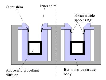
Figure 1-3: Cross-section view of the thruster with shim electrodes and main anode.
