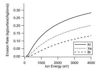
Figure A-5: Erosion Rate of Carbon per kilogram of bismuth, xenon, and krypton ions
