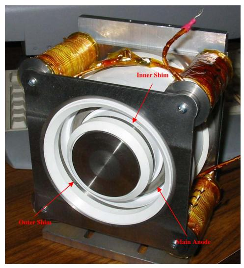
Figure 2-3: Photograph of the segmented electrode hall thruster
