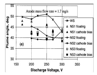
Figure 1-6: Observed changes in plume divergence for several segmented electrode configurations, from Ref. 18
