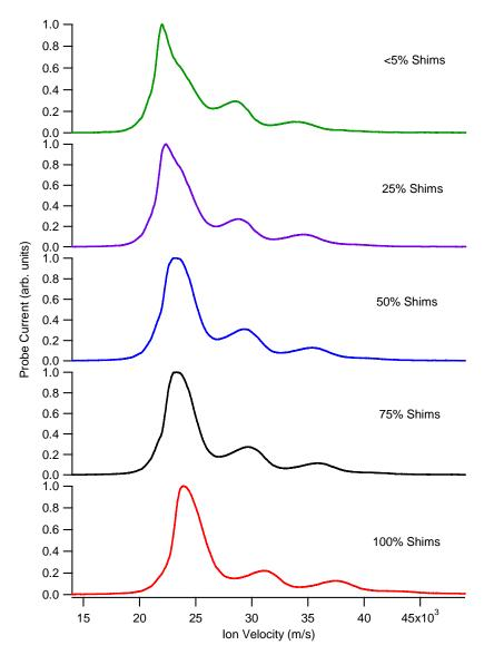
Figure 6-21: ExB probe traces taken as the level of shim current was varied. Data are for 400 V on the anode and 6 mg/s of xenon
