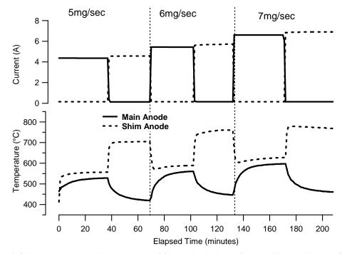
Figure 1-4: Temperature and current deposition on both the main and shim anodes as a function of time for a thruster operating at 400 V
