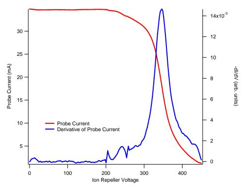
Figure 5-4: Typical RPA I-V sweep and associated derivative of current with respect to voltage, with 350 V on the anode, 5 mg/s of propellant flow, and all discharge heating on the shims.
