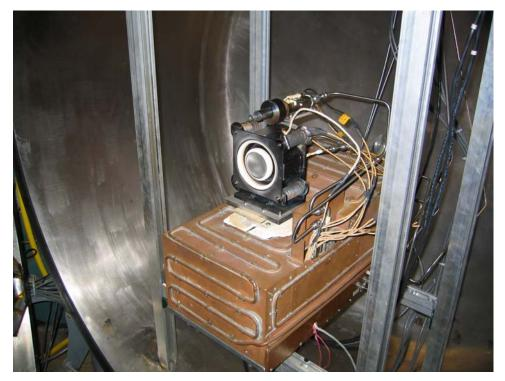
Figure 3-3: Photograph of a Hall thruster on the thrust stand
