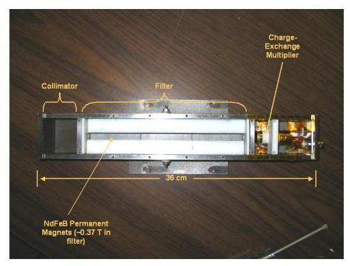
Figure 6-4: Photograph of the ExB probe with the top plate removed
