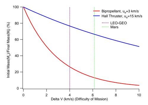
Figure 1-1: Mass Ratios as a function of mission  $\Delta v$  for a chemical rocket and a Hall thruster
