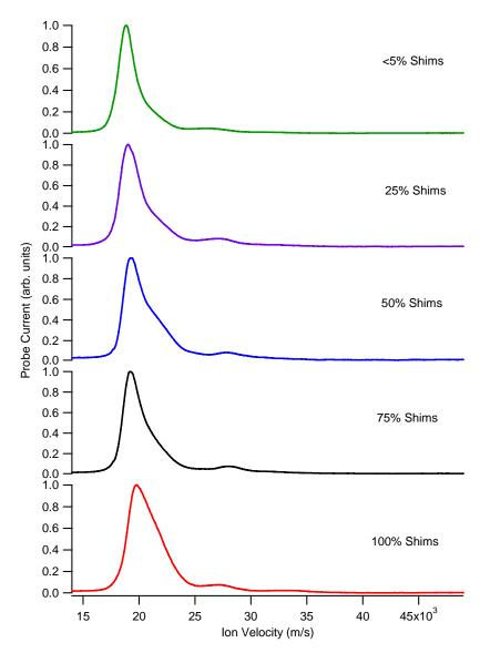
Figure 6-14: ExB probe traces taken as the level of shim current was varied. Data are for 300 V on the anode and 5 mg/s of xenon
