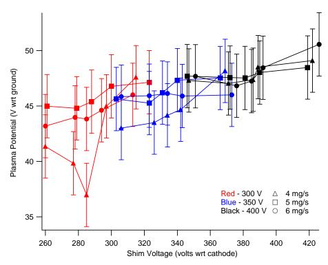
Figure 5-6: Plasma Potential relative to ground as a function of all three experimental factors, measured on the axis of the thruster, 500 mm from the exit plane.
