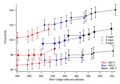
Figure 3-10: Thrust measured as a function of all three experimental factors. Higher shim voltages for a given mass flow and anode voltage combination correspond to higher discharge heating acceptance by the shims.
