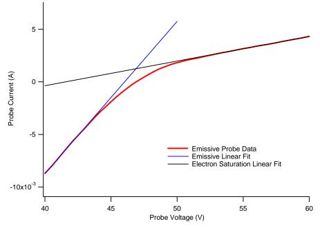
Figure 5-5: Typical emissive probe trace
