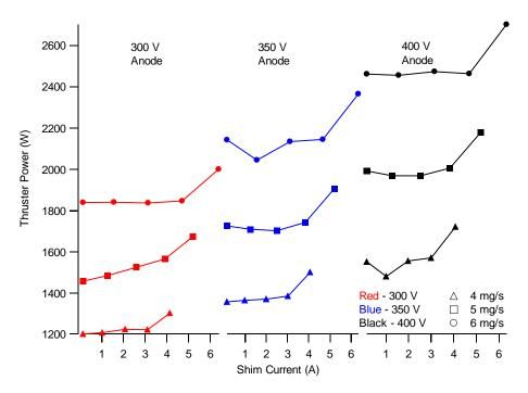
Figure 3-9: Discharge power as a function of all three experimental factors **Thrust Characterization**
