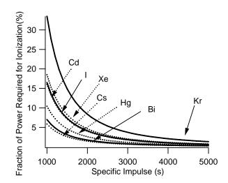
Figure A-2: Fraction of thruster power required for ionization vs. Isp for all propellants examined
