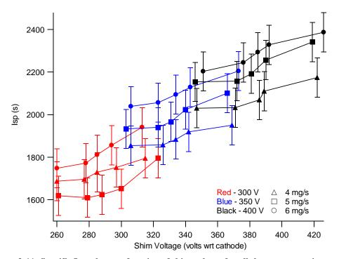
Figure 3-11: Specific Impulse as a function of shim voltage for all thruster operating conditions tested. Higher shim voltage for a given anode voltage indicates higher discharge electron heating on the shims.
