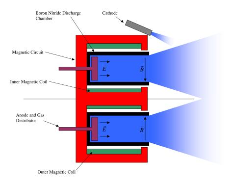
Figure 1-2: Cross Sectional View of a typical Hall thruster
