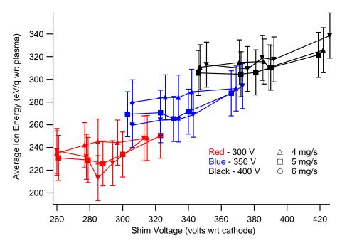
Figure 5-11: Average ion energy as a function of all three experimental factors. Higher shim voltage for a given combination of anode voltage and mass flow indicates higher discharge heating on the shims
