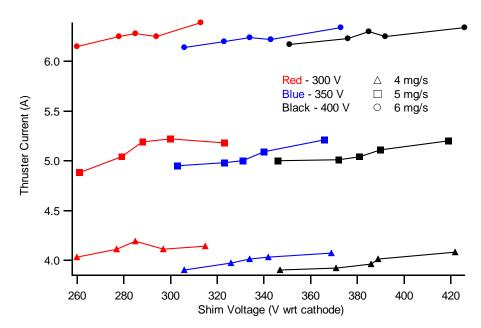
Figure 3-8: Total thruster current as a function of all three experimental factors
