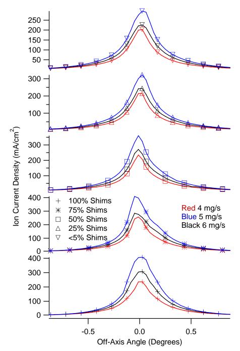
Figure 4-3: Beam Profiles with 350 V on the anode at all mass flows and levels of discharge current heating
