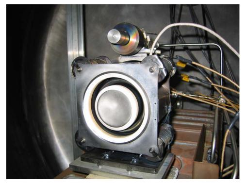
Figure 2-1: Photograph of the BPT-2000 with cathode
