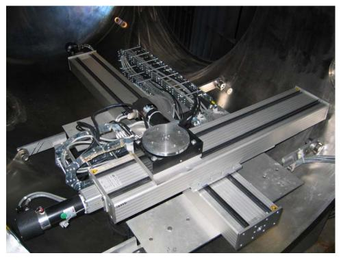
Figure 3-2: Photograph of the motion control table inside the XTF
