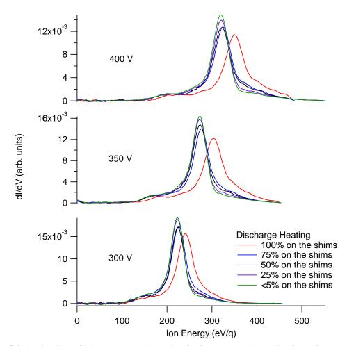
Figure 5-9: Derivatives of RPA current with at 6 mg/s of xenon, at all combinations of anode voltages and shim levels
