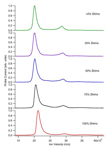
Figure 6-17: ExB probe traces taken as the level of shim current was varied. Data are for 350 V on the anode and 5 mg/s of xenon
