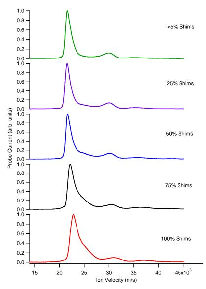
Figure 6-16: ExB probe traces taken as the level of shim current was varied. Data are for 350 V on the anode and 4 mg/s of xenon
