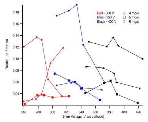
Figure 6-10: Doubly charged ion density fraction for all thruster operating points examined. High shim voltages indicate high amounts of discharge current attachment on the shims
