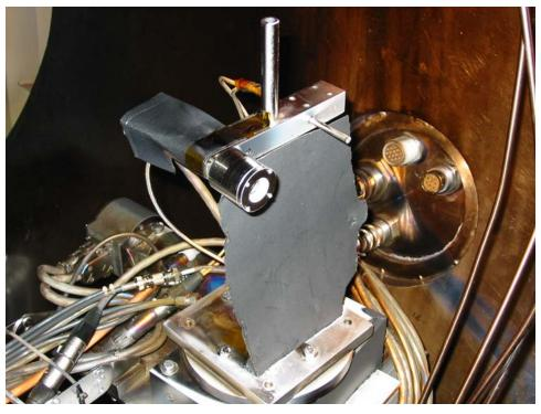
Figure 5-3: Photograph of an RPA in the vacuum facility
