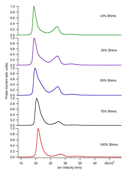
Figure 6-15: ExB probe traces taken as the level of shim current was varied. Data are for 300 V on the anode and 6 mg/s of xenon
