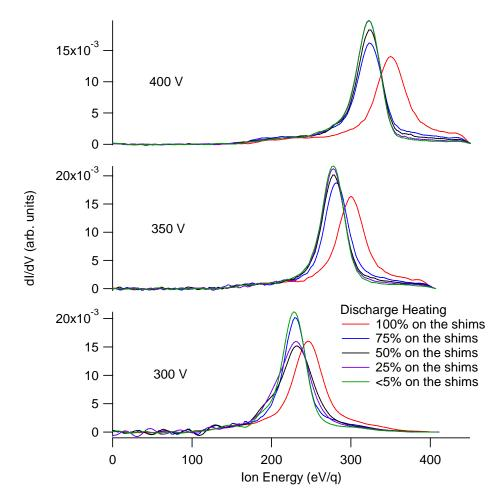
Figure 5-7: Derivatives of RPA current with at 4 mg/s of xenon, at all combinations of anode voltages and shim levels
