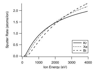
Figure A-4: Sputter Yield of carbon under bismuth, xenon and krypton ion collisions
