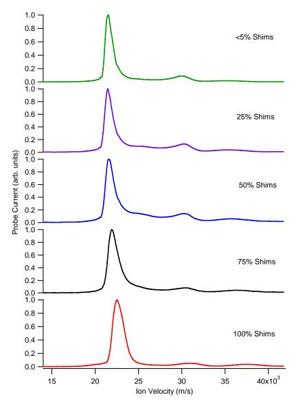
Figure 6-20: ExB probe traces taken as the level of shim current was varied. Data are for 400 V on the anode and 5 mg/s of xenon
