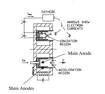
Figure 1-5: Diagram of a two-stage Hall thruster as used in Ref. 8
