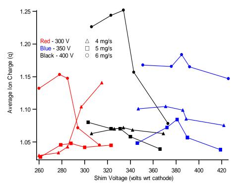
Figure 6-12: Average ion charge as a function of all three experimental factors. High shim voltage for indicates a higher fraction of discharge current heating on the shims.
