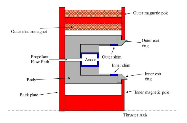
Figure 2-4: Cross section of the segmented anode thruster
