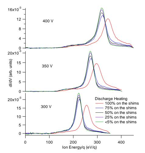
Figure 5-8: Derivatives of RPA current with at 5 mg/s of xenon, at all combinations of anode voltages and shim levels
