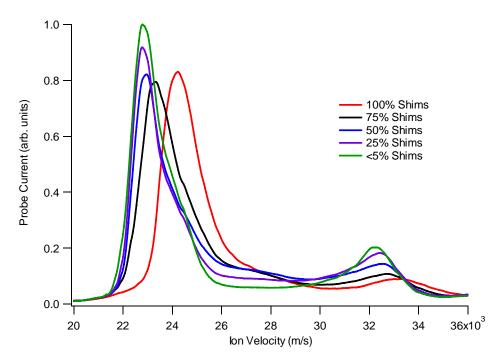
Figure 6-8: ExB probe traces taken with 400 V on the main anode and 4 mg/s of xenon.
