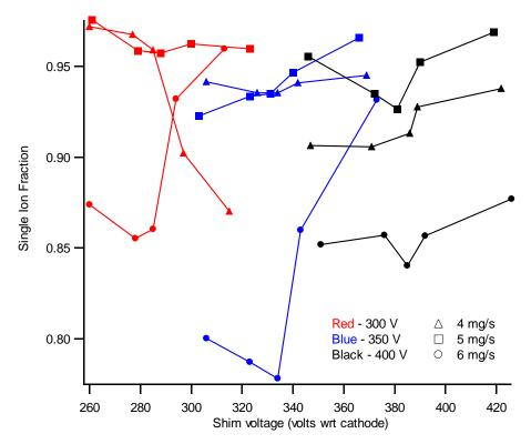
Figure 6-9: Singly charged ion density fraction for all thruster operating points examined. High shim voltages indicate high amounts of discharge current attachment on the shims
