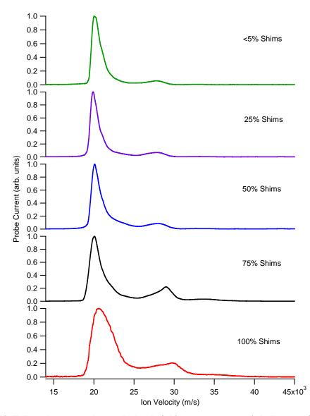
Figure 6-13: ExB probe traces taken as the level of shim current was varied. Data are for 300 V on the anode and 4 mg/s of xenon
