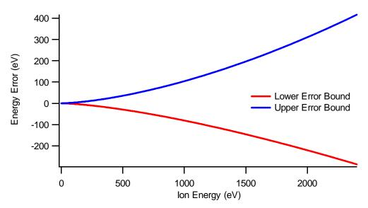
Figure 6-5: Resolution error of the ExB probe as a function of ion energy
