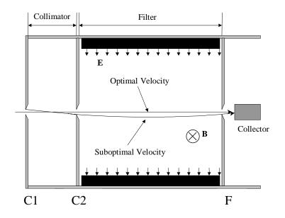
Figure 6-3: Schematic view of ExB probe showing detection of an off-axis ion. Plate C1 is the front plate of the probe, C2 is the filter entry or collimator exit plate, and F is the filter exit plate.
