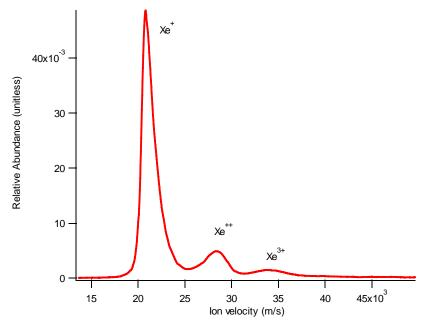
Figure 6-2: Typical normalized ExB probe distribution
