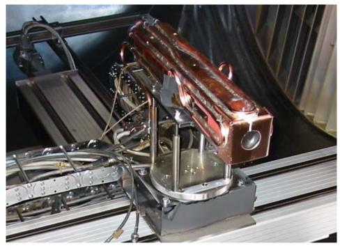
Figure 6-6: Photograph of the ExB probe in the water-cooled shroud
