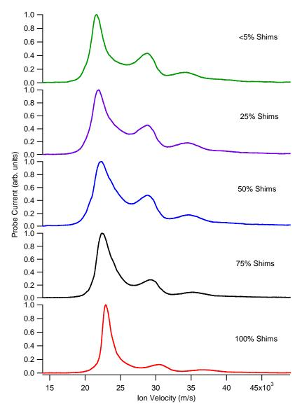
Figure 6-18: ExB probe traces taken as the level of shim current was varied. Data are for 350 V on the anode and 6 mg/s of xenon
