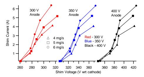
Figure 3-7: Shim Current as a function of shim voltage at all thruster operating points
