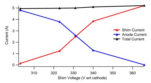
Figure 3-6: Characteristic shift in current on the shims and main anode as shim voltage was varied. Thruster was operating at 350 V on the anode and 5 mg/s of mass flow.
