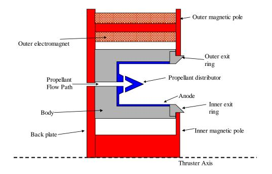
Figure 2-2: Cross section of the BPT-2000 Hall thruster
