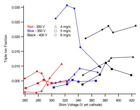
Figure 6-11: Triply charged ion density fraction for all thruster operating points examined. High shim voltages indicate high amounts of discharge current attachment on the shims
