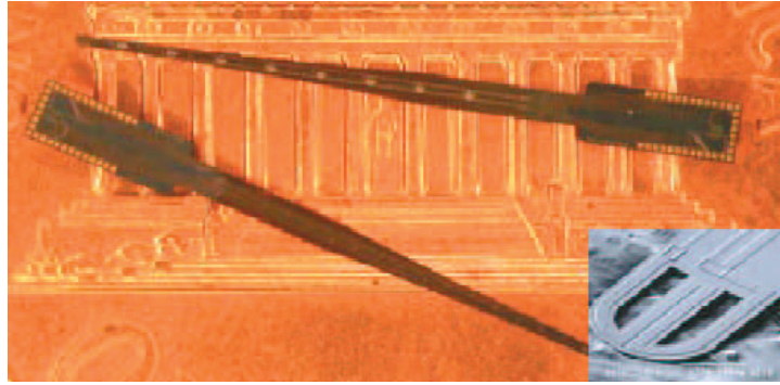
Figure 3.3 Probe level piezoresistive strain gages & tip sensor (inset) [27].
