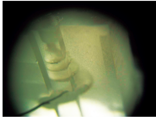
Figure 4.19 Insertion test for a 3x single-chambered device into an acrylic ST model [32].
