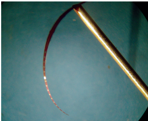
Figure 4.5 Silicon probe with wrongly directed curvature.
