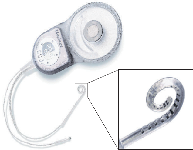
Figure 1.6 Cochlear Corporation's Nucleus 24 Contour Implant with pre-curved electrode array (inset) [16].
