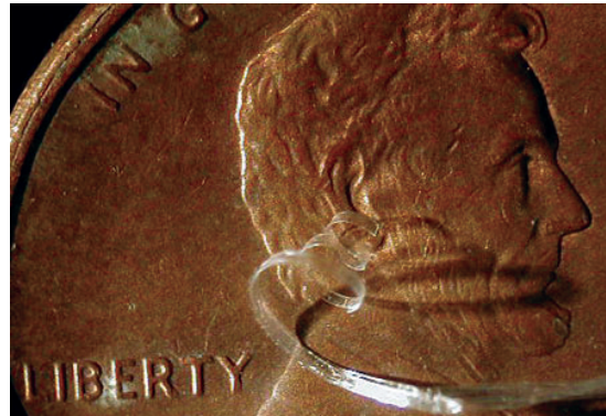
Figure 4.15 A 1x three chambered insertion tool.
