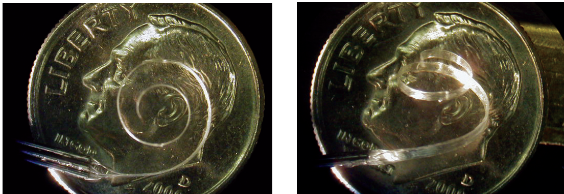
Figure 4.11 Two views of a 3x, three chambered insertion tool.
