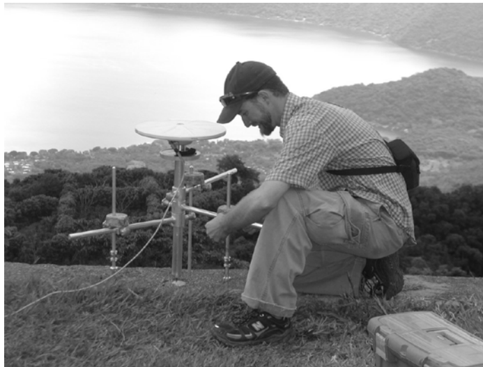
Tripod setup. A fixed elevation tripod with precise leveling can be assembled and by one person and practically eliminates setup error. Photo by author.
