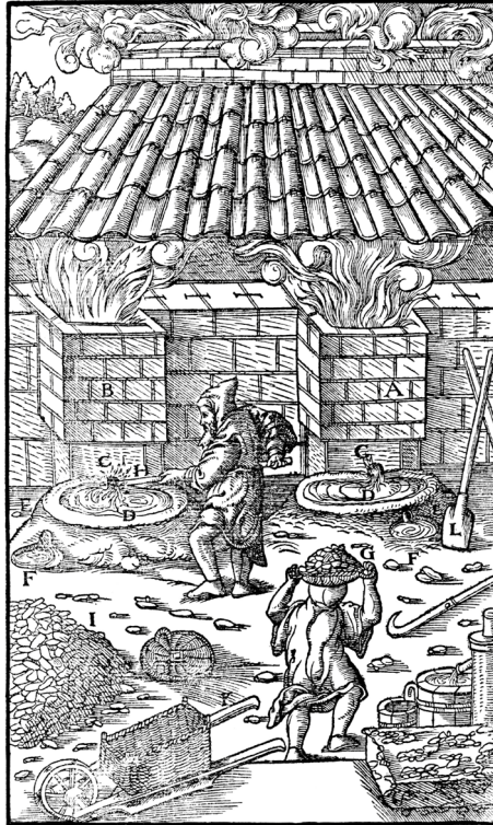
Figure 2.6 German smelting ca. 1550s. Note similarities to the late Bronze Age furnace in Figure 2.4. Except for stack height and the arrangement of the furnaces to better use water power for air blasts, the process appears little changed. (After Agricola 1950, 389.)
