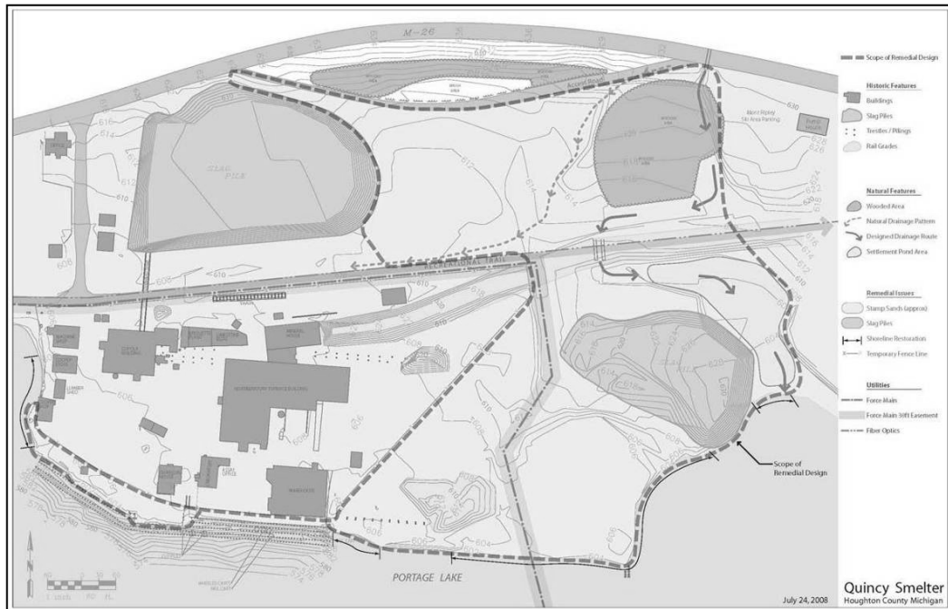
Figure 7.6 Quincy Smelter Base map for proposed final remediation 2009. The area inside the dashed lines will be graded, covered with soil, and vegetated to arrest erosion. The slag plies (b) will be left alone but some passive restraint will be erected, such as a short fence. The arrows indicate new water drainage from the hillside. The buildings will not receive any further remediation treatment beyond the asbestos removal of 2008. (Source: EPA, Proposed Plan for Record of Decision Amendment for Operable Unit 3 at Torch Lake Superfund Site, 5)
