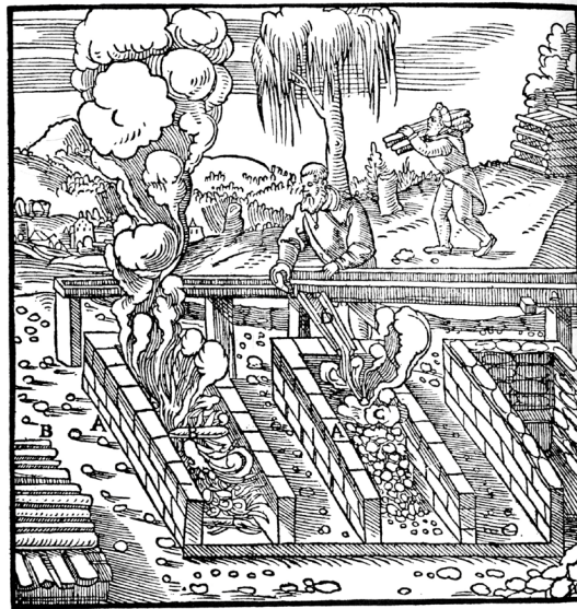
Figure 2.5 German multiple-bin ore roasting ca. 1550. (After Agricola 93 1950, 350)
