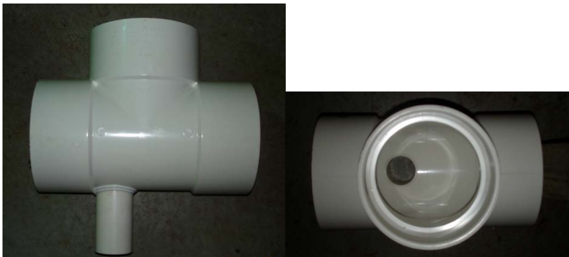
Figure 8. Photo of the fabricated PVC fitting (8" size) used for stilling well installation in existing pipe at the Gainesville site (profile – left, aerial – right).
