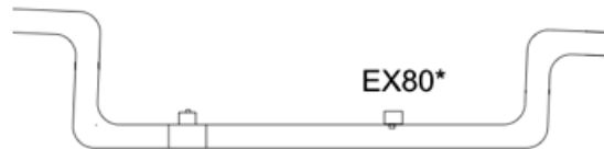
Figure 4. Line modification measurement system (trap system) that creates full pipe conditions and utilizes a measurement technology such as the Global Water EX80 electromagnetic meter as pictured here. A cleanout is included in the design. Flow is from left to right.
