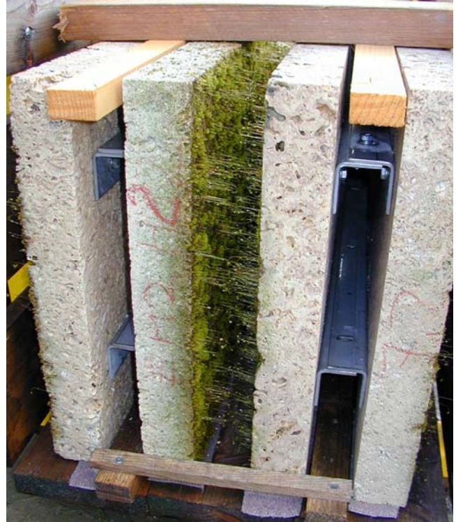
Figure 49. These mosses are being cultured on tufa to be used in building construction. Photo courtesy of Michel Chiaffredo.
