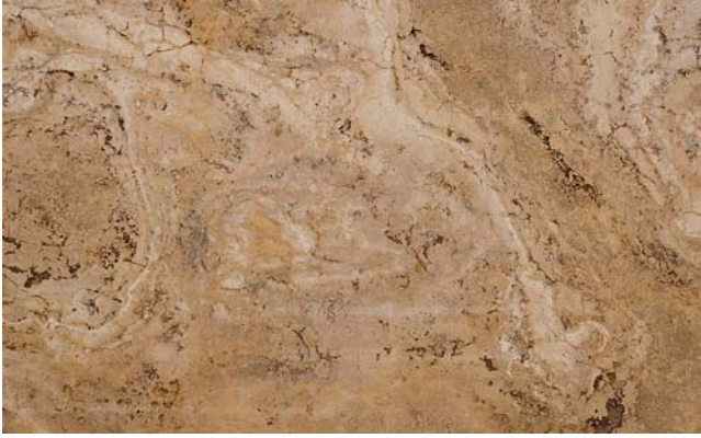
Figure 29. Travertine facade sample for wall. Photo by Julian Herzog, through Creative Commons.
