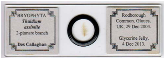
Figure 21. Slide labels using a laser printer, PVA glue, and hair lacquer. Photo by Des Callaghan.
