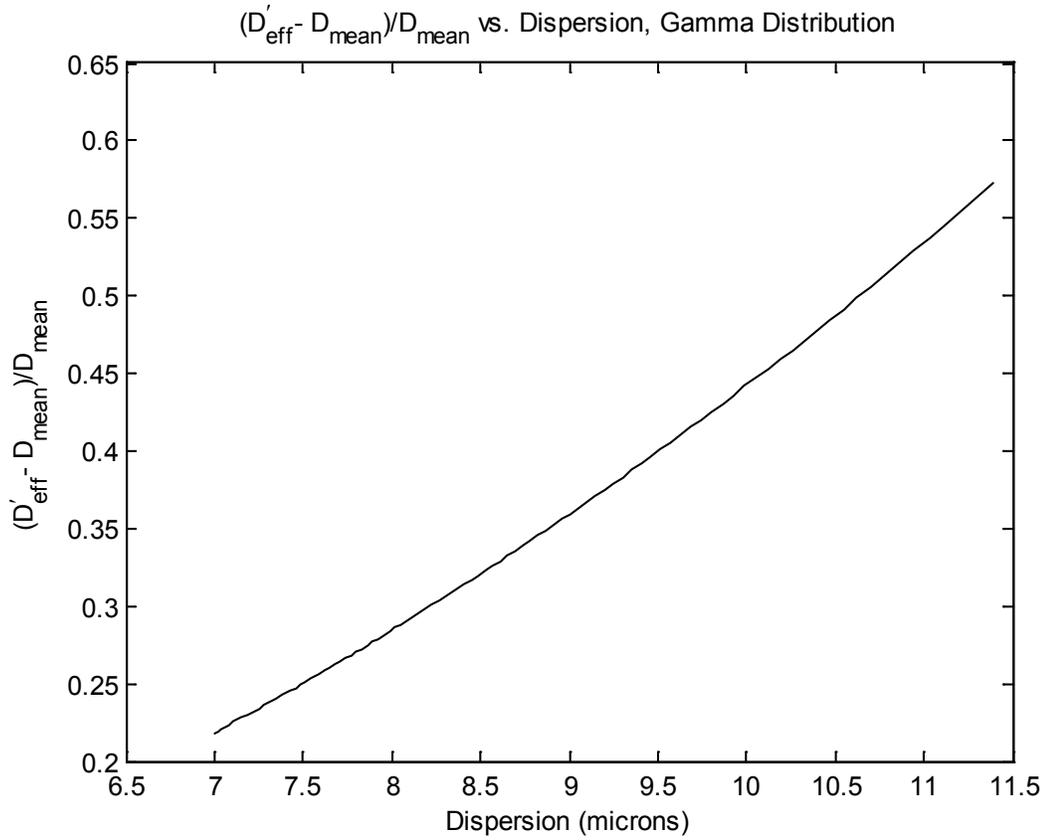
Figure 3.3: At a constant mean of  $27.9 \mu\text{m}$ , as the dispersion ( $\sigma = (Cb)^{1/2}$ ) increases, the normalized difference between the lidar-radar effective diameter and the mean increases. The scale parameter ( $b$ ) varies between 1.8 and 4.7.
