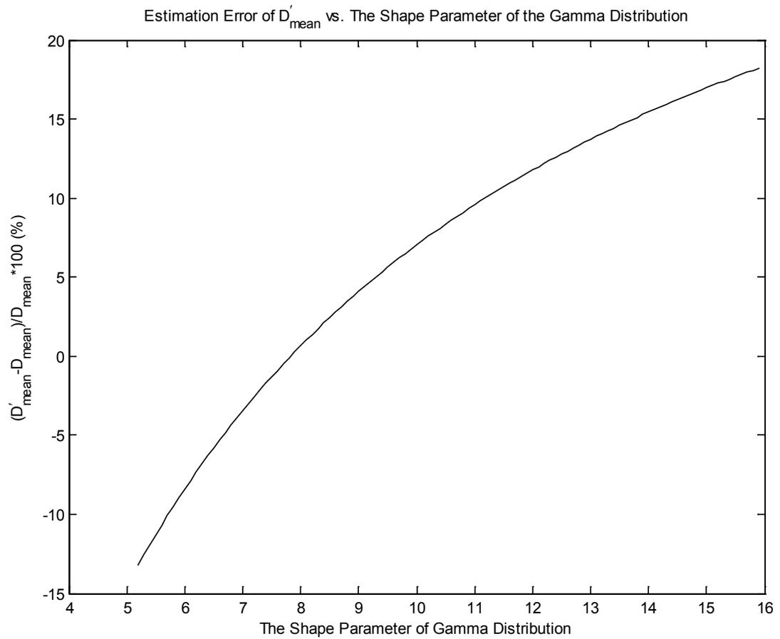
*Figure 4.2: Using the lidar-radar effective diameter of the 87,000 laboratory drops and the shape parameter range of 5.2 to 15.9 from Miles et al. (2000), we show the estimation error of the lidar-radar mean diameter as a function of gamma distribution shape parameters.*
