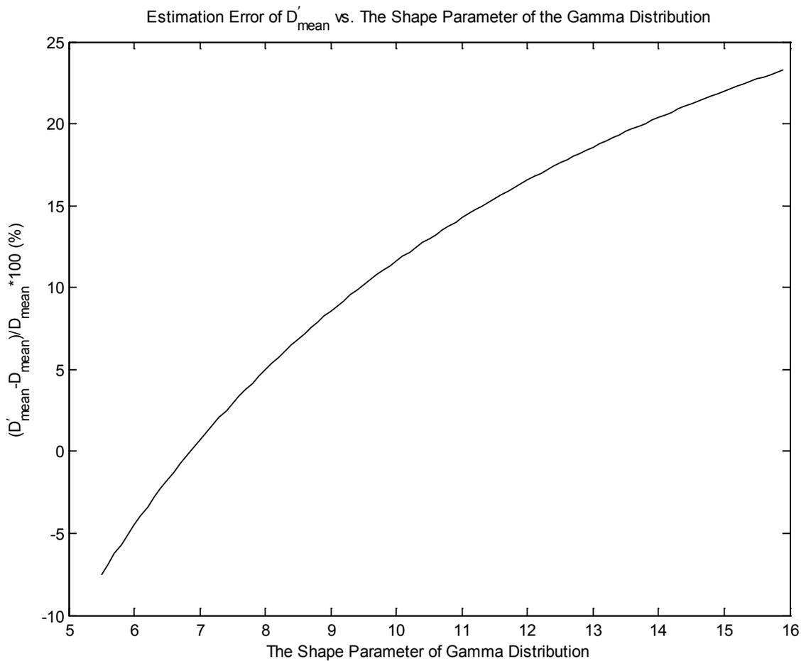
*Figure 5.2: Using the lidar-radar effective diameter derived from the random sampling of the cumulative distribution function in Figure 4.1.1 and the shape parameter range of 5.5 to 15.9 given Miles et al. (2000), we show the estimation error of the lidar-radar mean diameter as a function of gamma distribution shape parameters.*
