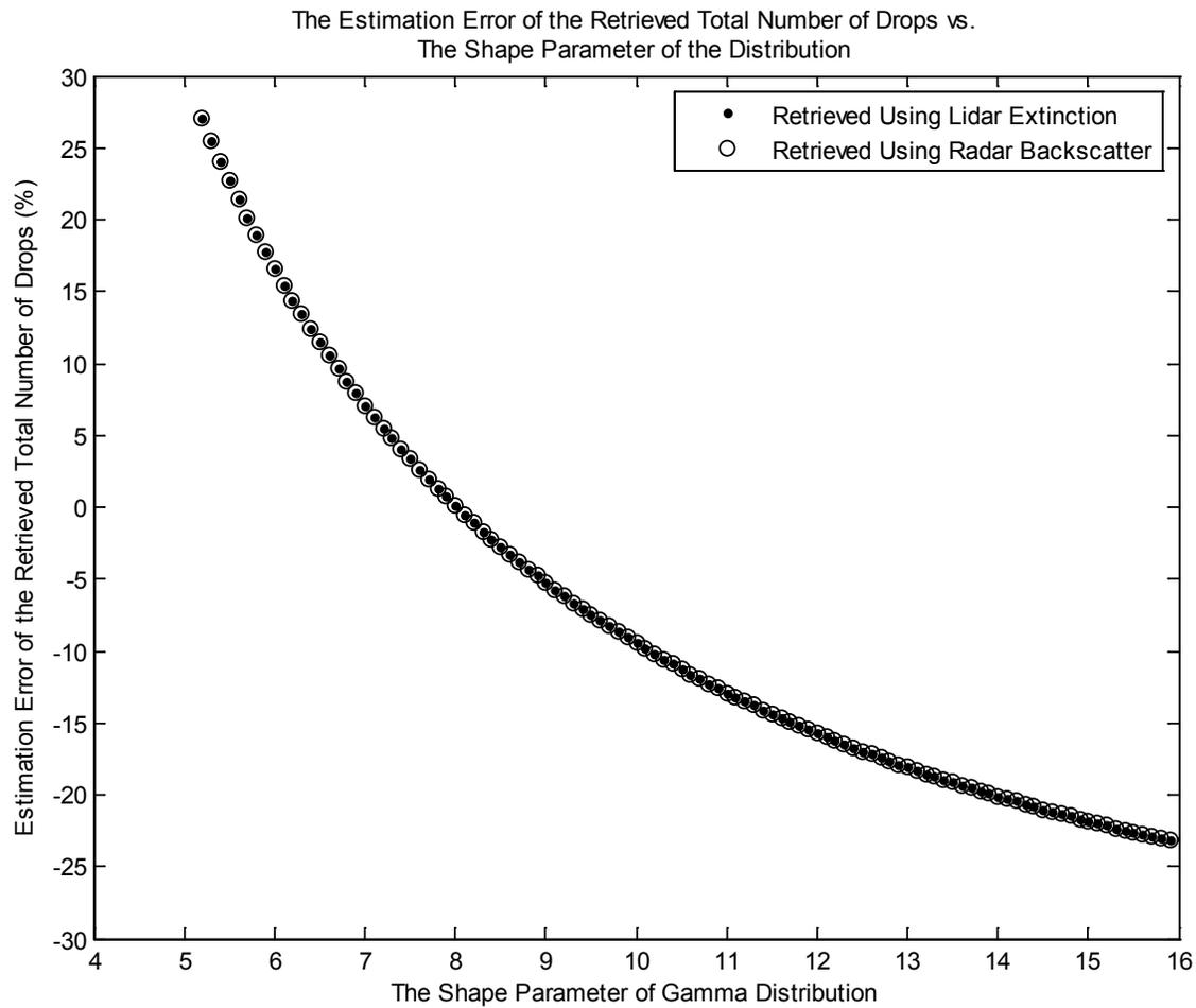
*Figure 4.3: Using the simulated scattering from 87,000 laboratory drops and the shape parameter range of 5.2 to 15.9 from Miles et al. (2000), we show the estimation error of the total number of drops as a function of gamma distribution shape parameters. The number of drops was computed using either the second moment of the distribution and the lidar extinction cross section (dots) or the sixth moment of the distribution and the radar backscatter cross section (circles).*
