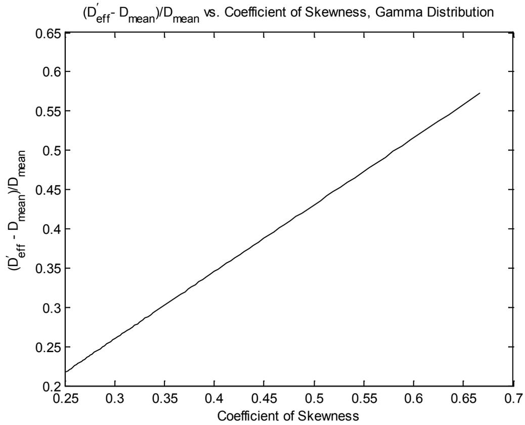
Figure 3.2: Varying the shape parameter (6 to 15.9) of the gamma distribution shows that as the coefficient of skewness ( $S = 2a^{-1/2}$ ) increases, the normalized difference between the lidar-radar effective diameter and the mean increases.
