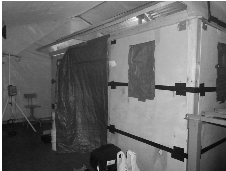
Figure 2.1: Kitchen 2.0 in the clean room. Tarps were used to cover the door and windows so they could be opened or closed easily. Note the gables at either end were always sealed during testing, and the eaves were sealed unless otherwise specified (photo credit: author).
