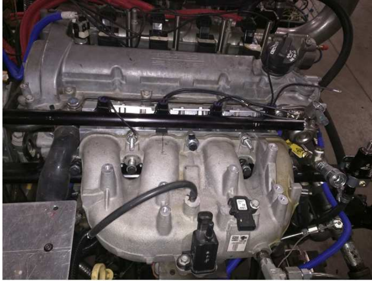
Figure B.1: Port fuel injectors installed and wired on the common rail.
