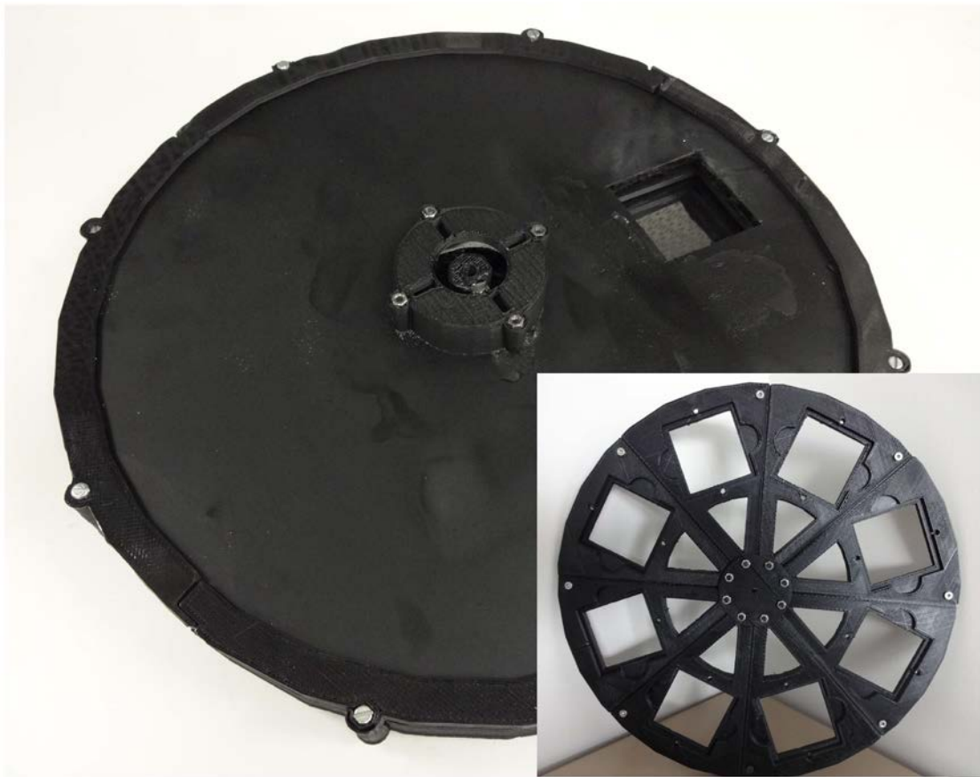
Figure 2.3.6. Automated filter wheel switcher
