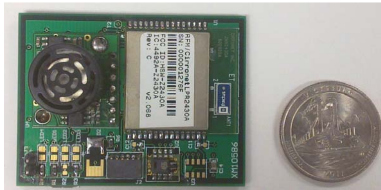
Figure 4.1: The static sensor node in CosNet. The front contains the ultrasonic transceiver, the networking module, a temperature sensor, and a photonic sensor.
