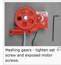
23. Remove the hobbled bolt and large gear to expose the remaining motor mounting screws and tighten them. Replace the large gear and hobbled bolt insuring that all the spacer washers are in place. Recheck hob position relative to filament path.
