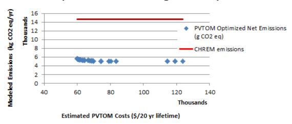
Figure 6. House B (Low thermal and high electric consumption) Pareto Front.
